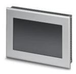
Touch panel with 17.8 cm/7" TFT-Display (Analog resistive), 800 x 480 Pixel (WVGA), 65536 colors, ARM9<sup>™</sup>, 200 MHz, 2x USB Host 2.0, 1 x Ethernet (10/100 Mbps), RJ45, Windows CE 5.0 and User software: MicroBrowser. (Bus system: without)
