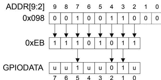
During a read, if the address bit associated with the data bit is set to 1, the value is read. If the address bit associated with the data bit is set to 0, it is read as a zero, regardless of its actual value. For example, reading address GPIODATA + 0x0C4 yields as shown in Figure 7-4 on page 235.
