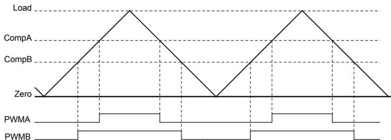
In this example, the first generator is set to drive High on match A up, drive Low on match A down, and ignore the other four events. The second generator is set to drive High on match B up, drive Low on match B down, and ignore the other four events. Changing the value of comparator A changes the duty cycle of the  $PWMA$  signal, and changing the value of comparator B changes the duty cycle of the  $PWMB$  signal.
