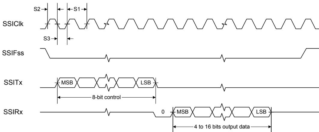
Figure 19-14. SSI Timing for SPI Frame Format (FRF=00), with SPH=1
