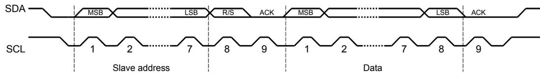
The first seven bits of the first byte make up the slave address (see Figure 13-5 on page 449). The eighth bit determines the direction of the message. A zero in the R/S position of the first byte means that the master will write (send) data to the selected slave, and a one in this position means that the master will receive data from the slave.
