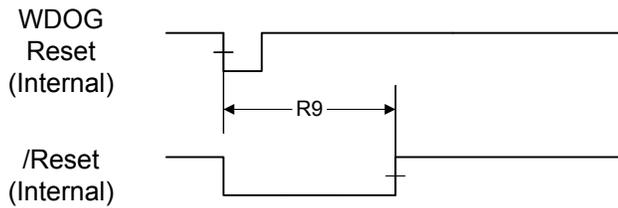
**Figure 19-10. LDO Reset Timing**
