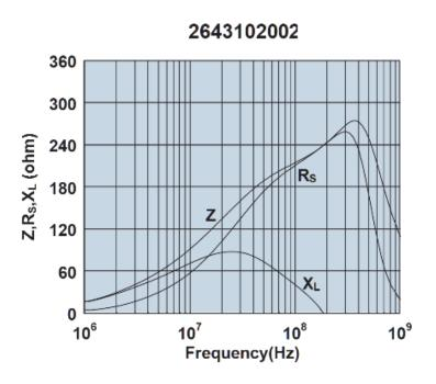
Impedance, reactance, and resistance vs. frequency.
