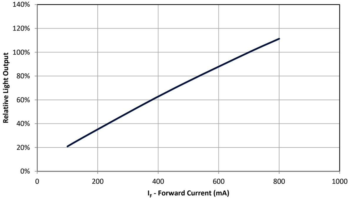
Figure 6: Typical relative light output vs. forward current @ T<sub>c</sub> = 25°C.
