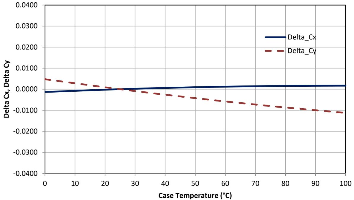
Figure 9: Typical chromaticity coordinate shift vs. Case temperature
