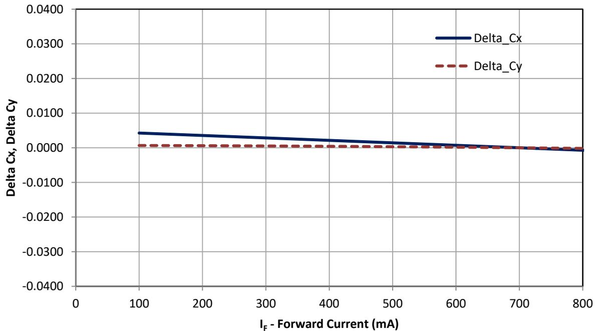
Figure 8: Typical chromaticity coordinate shift vs. forward current
