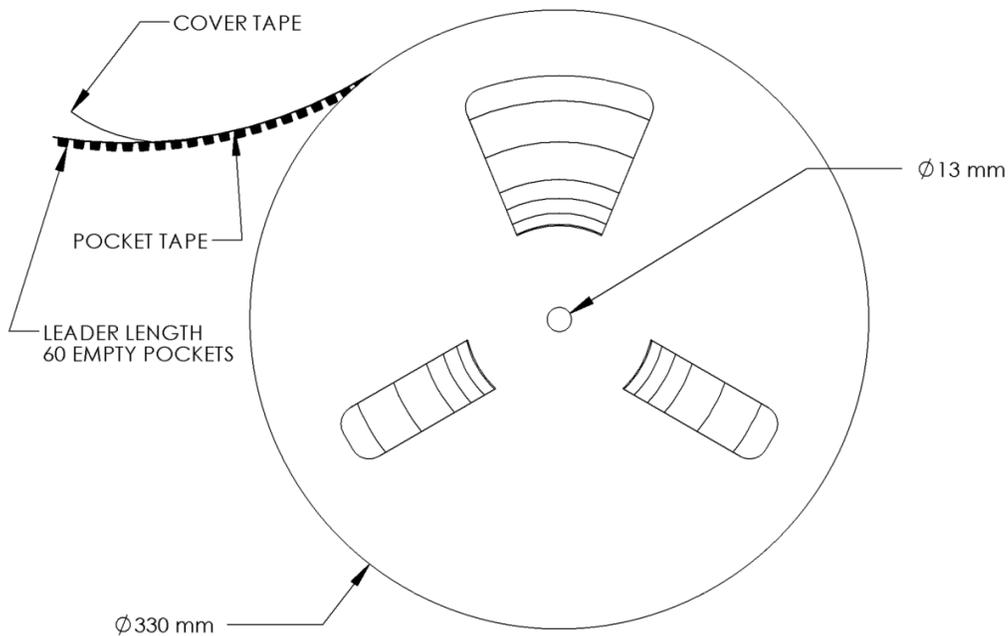
Figure 13: Emitter Reel specifications (mm).
