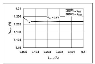
**FIGURE 2-11:** V<sub>OUT1</sub> vs. I<sub>OUT1</sub> (V<sub>OUT1</sub> = 1.2V).
