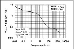
FIGURE 2-35: V<sub>OUT2</sub> Noise vs. Frequency.
