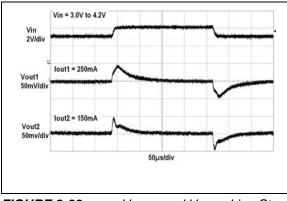
**FIGURE 2-38:** V<sub>OUT1</sub> and V<sub>OUT2</sub> Line Step Response vs. Time.
