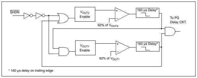
FIGURE 4-2: TC1304 Sequencing Circuit.
