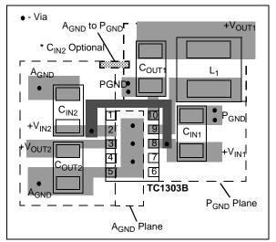
FIGURE 5-2: Component Placement, Fixed 10-Pin DFN.
