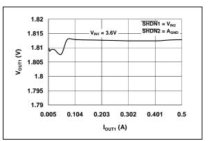
**FIGURE 2-12:** V<sub>OUT1</sub> vs. I<sub>OUT1</sub> (V<sub>OUT1</sub> = 1.8V).
