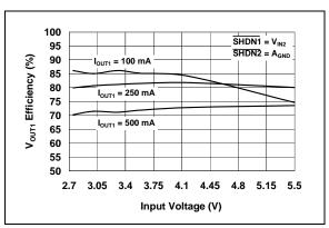
**FIGURE 2-5:**  $V_{OUT1}$  Output Efficiency vs. Input Voltage ( $V_{OUT1} = 1.2V$ ).
