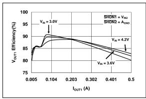
**FIGURE 2-8:**  $V_{OUT1}$  Output Efficiency vs.  $I_{OUT1}$  ( $V_{OUT1} = 1.8V$ ).
