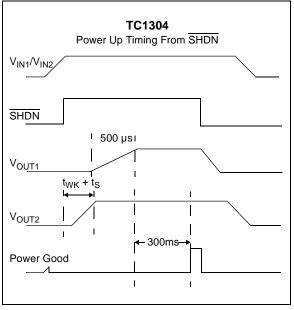
FIGURE 4-3: TC1304 Power-up Timing from SHDN.
