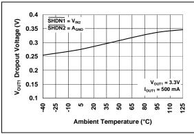
*FIGURE 2-19:* V<sub>OUT1</sub> Dropout Voltage vs. Ambient Temperature.
