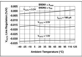
**FIGURE 2-28:** V<sub>OUT2</sub> Line Regulation vs. Ambient Temperature.
