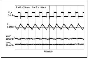
**FIGURE 2-20:** V<sub>OUT1</sub> and V<sub>OUT2</sub> Heavy Load Switching Waveforms vs. Time.
