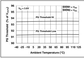
*FIGURE 2-31:* PG Threshold Voltage vs. Ambient Temperature.
