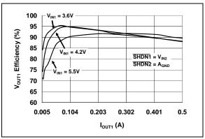
**FIGURE 2-10:**  $V_{OUT1}$  Output Efficiency vs.  $I_{OUT1}$  ( $V_{OUT1} = 3.3V$ ).
