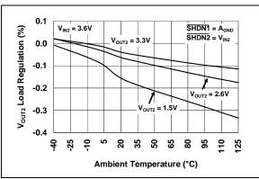
**FIGURE 2-29:** V<sub>OUT2</sub> Load Regulation vs. Ambient Temperature.
