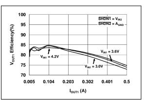
**FIGURE 2-6:**  $V_{OUT1}$  Output Efficiency vs.  $I_{OUT1}$  ( $V_{OUT1} = 1.2$  V).
