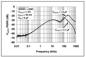
FIGURE 2-34: V<sub>OUT2</sub> Power Supply Ripple Rejection vs. Frequency.
