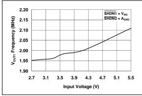
**FIGURE 2-14:** V<sub>OUT1</sub> Switching Frequency vs. Input Voltage.
