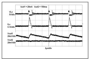
**FIGURE 2-21:** V<sub>OUT1</sub> and V<sub>OUT2</sub> Light Load Switching Waveforms vs. Time.
