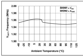
FIGURE 2-15: V<sub>OUT1</sub> Switching Frequency vs. Ambient Temperature.
