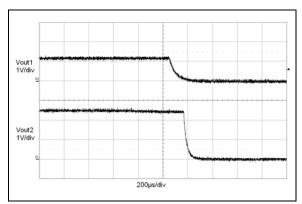
FIGURE 2-43: Shutdown Waveforms (TC1304).
