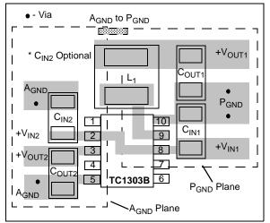
FIGURE 5-1: Component Placement, Fixed 10-Pin MSOP.
