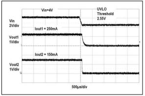
V<sub>OUT1</sub> and V<sub>OUT2</sub> Shutdown FIGURE 2-40: Waveforms.
