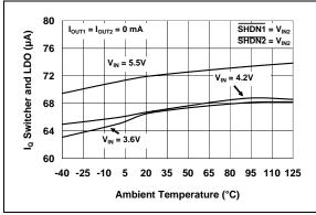
**FIGURE 2-1:** I<sub>Q</sub> Switcher and LDO Current vs. Ambient Temperature (TC1303A,B).
