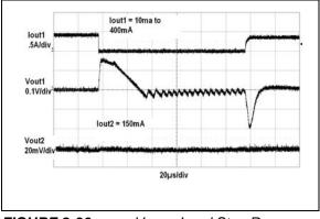
FIGURE 2-36: V<sub>OUT1</sub> Load Step Response vs. Time.
