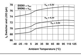
**FIGURE 2-2:** I<sub>Q</sub> Switcher and LDO Current vs. Ambient Temperature (TC1303C, TC1304).
