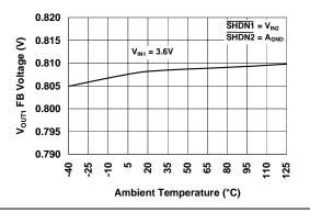
**FIGURE 2-16:** V<sub>OUT1</sub> Adjustable Feedback Voltage vs. Ambient Temperature.
