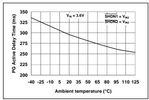
FIGURE 2-30: PG Active Delay Time-out vs. Ambient Temperature.
