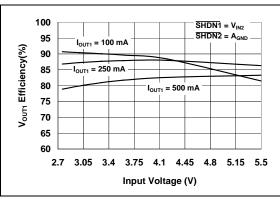
**FIGURE 2-7:**  $V_{OUT1}$  Output Efficiency vs. Input Voltage ( $V_{OUT1} = 1.8V$ ).
