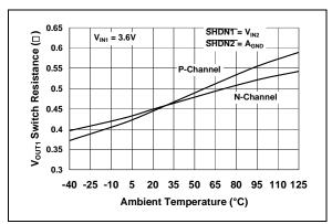
**FIGURE 2-18:** V<sub>OUT1</sub> Switch Resistance vs. Ambient Temperature.
