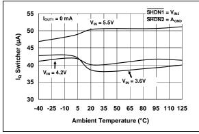
**FIGURE 2-3:** I<sub>Q</sub> Switcher Current vs. Ambient Temperature.
