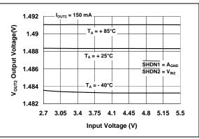
**FIGURE 2-22:**  $V_{OUT2}$  Output Voltage vs. Input Voltage ( $V_{OUT2} = 1.5V$ ).
