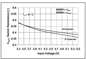
**FIGURE 2-17:** V<sub>OUT1</sub> Switch Resistance vs. Input Voltage.
