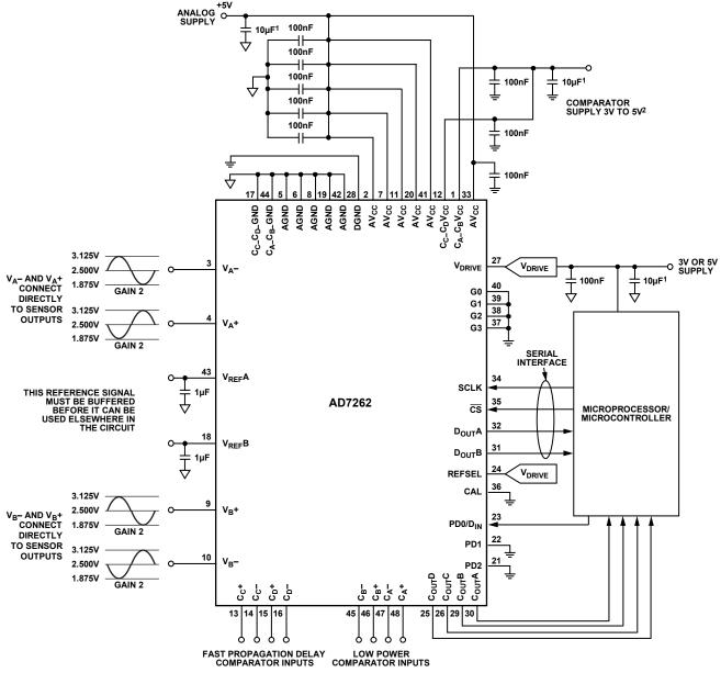
$^1\text{THESE}$  CAPACITORS ARE PLACED AT THE SUPPLY SOURCE AND MAY NOT BE REQUIRED IN ALL SYSTEMS.  $^2\text{THIS}$  SUPPLY CAN BE CONNECTED TO THE ANALOG 5V SUPPLY IF REQUIRED.
