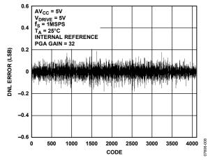
Figure 8. Typical DNL at Gain of 32
