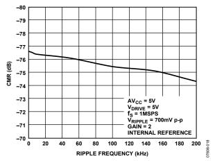
Figure 18. Common-Mode Rejection vs. Common-Mode Ripple Frequency
