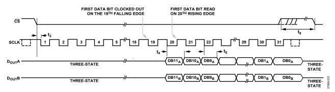
$\textit{Figure 33. Serial Interface Timing Diagram When Reading Data on the 20$^{th} \textit{Rising SCLK Edge with a 40 MHz SCLK}$}$
