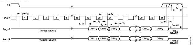
Figure 2. Serial Interface Timing Diagram
