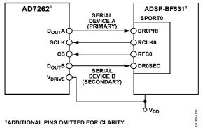
Figure 37. Interfacing the AD7262 to the ADSP-BF531
