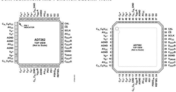
Figure 3. 48-Lead LQFP Pin Configuration
