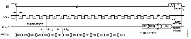
Figure 30. Timing Diagram for a Write Operation to the Control Register
