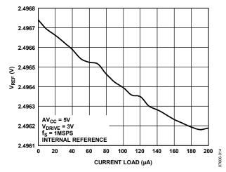
Figure 14. V<sub>REF</sub> vs. Reference Output Current Load
