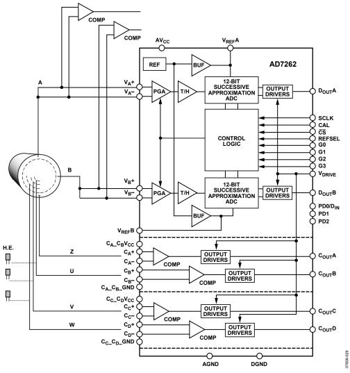
Figure 29. Typical System Connection Diagram with Optical Encoder
