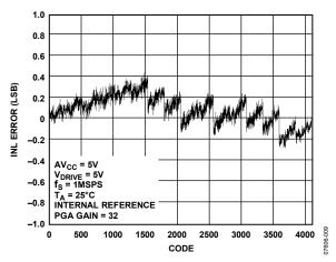
Figure 9. Typical INL at Gain of 32
