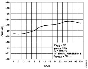
Figure 17. Common-Mode Rejection vs. Gain
