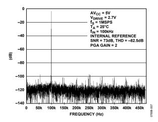
Figure 7. 3 dB Typical FFT at Gain of 2
