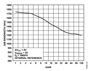
Figure 15. 3 dB Bandwidth vs. Gain
