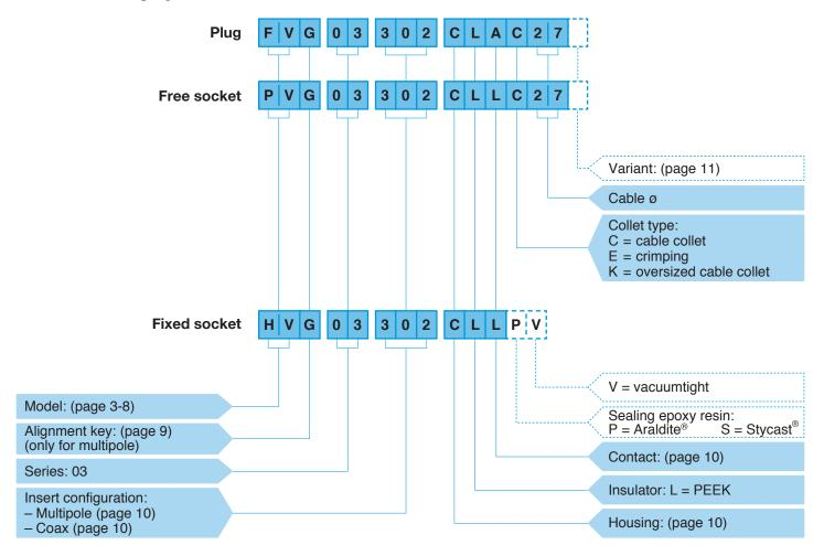
**FVG.03.302.CLAC27** = straight plug with key (G) and cable collet, 03 series, multipole type with 2 contacts, outer shell in chrome-plated brass, PEEK insulator, male solder contacts, C type collet for 2.7 mm diameter cable.
