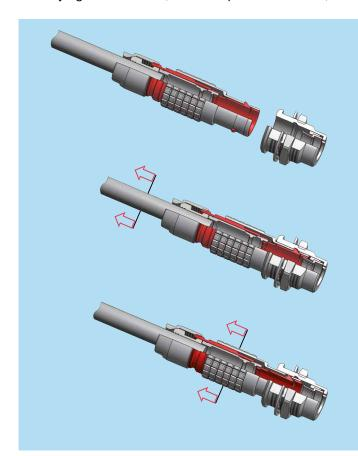
The LEMO self-latching system allows the connector to be mated by simply pushing the plug axially into the socket.
