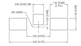
\*UNLESS OTHERWISE SPECIFIED TOLERANCES PER DECIMAL PRECISION ARE: X=±1 (±0.039), X.X=±0.5 (±0.020), X.XX=±0.25 (±0.010), X.XXX=±0.127 (±0.005). LEAD SIZE=±0.05 (±0.002), LEAD LENGTH=±0.75 (±0.030). MIN =  $\frac{+0.00}{-0.00}$  UNCONTROLLED DOCUMENT
