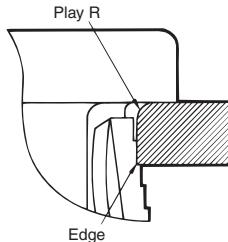
When processing the panel, be sure that the Play R is on the switch operation side. Be sure that the Edge is on the reverse side of panel when processing.
