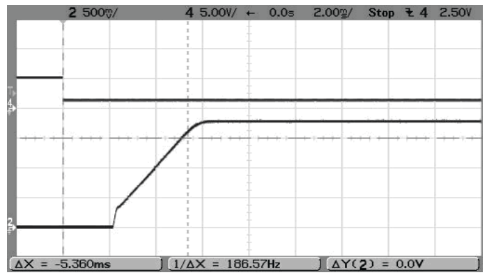
On/Off Enable Startup (V in =5V, V out =1.8V, I out =6A, Cload=0) Trace 4=Enable, Trace 2=V out
