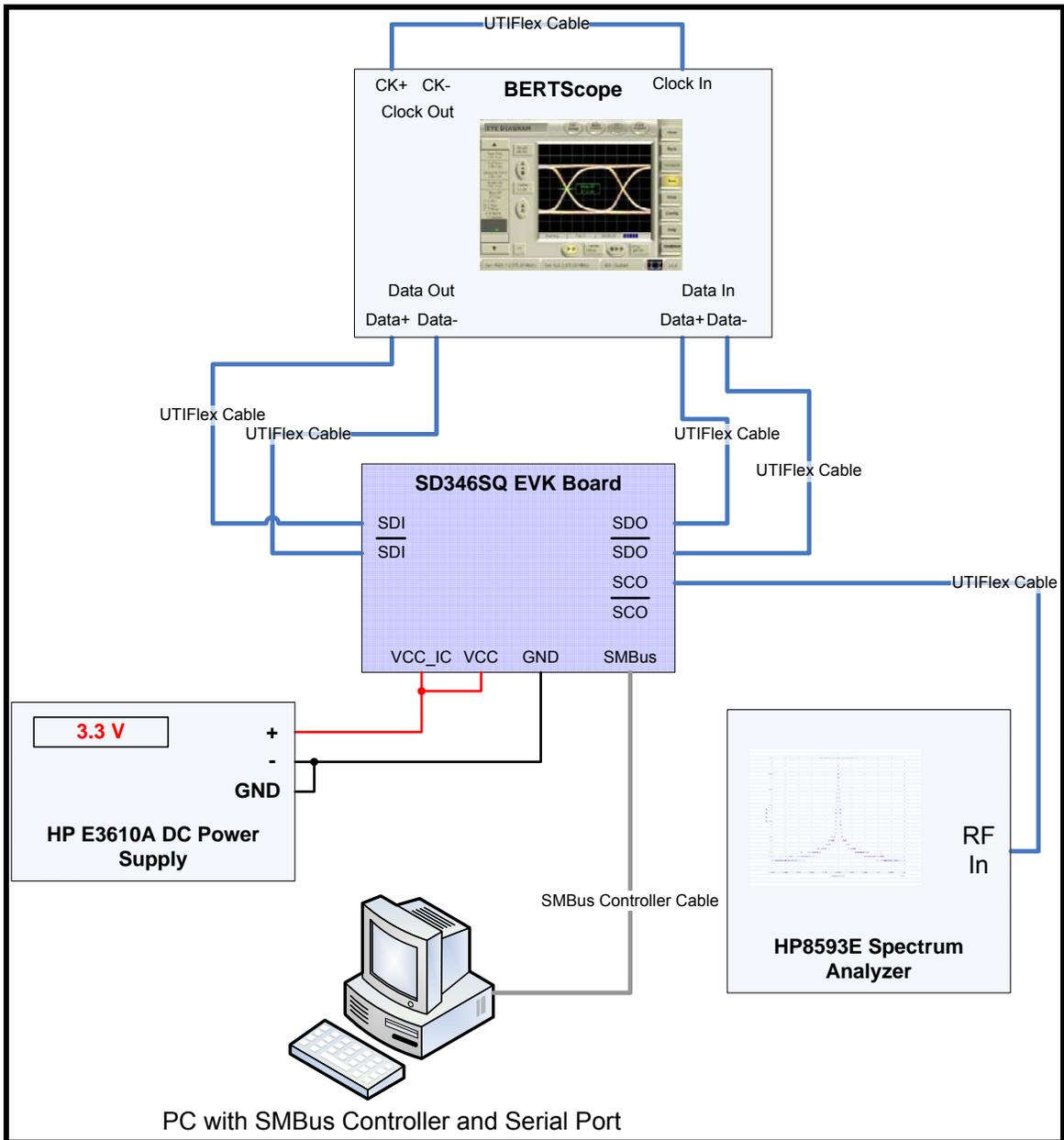
**Figure 2. Test setup for the SD346EVK board.**
