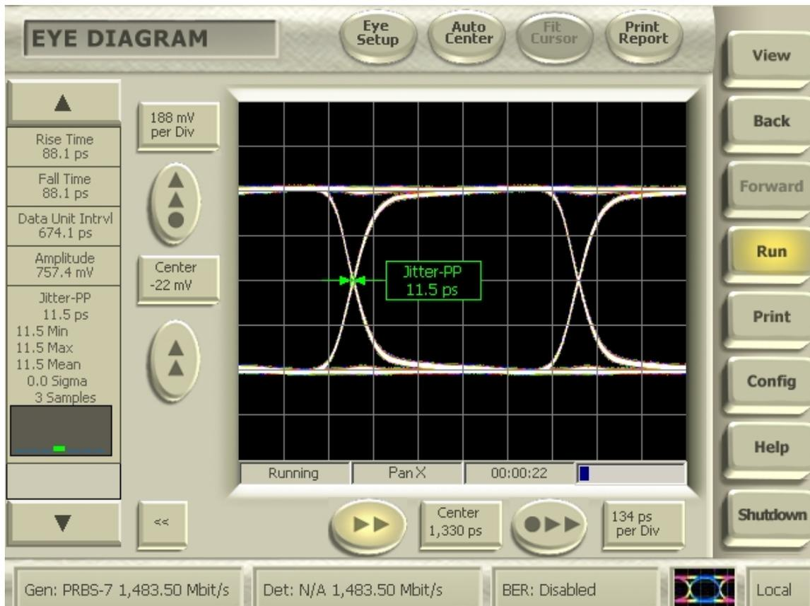
Figure 3. Typical output eye diagram for 1.4835 Gb/s.
