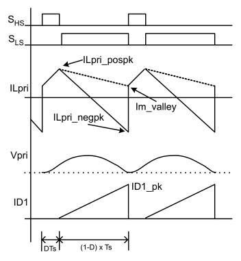
Figure 21. Simplified Voltage and Current Waveforms
