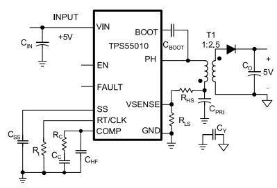
Figure 22. 5 V to 5 V Isolated Power Supply Schematic
