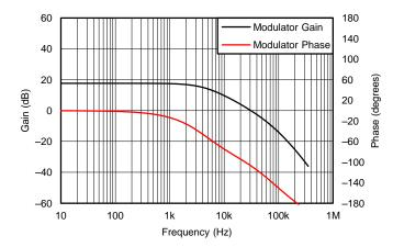
Figure 23. Modeled Modulator Small Signal Response
