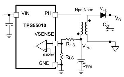
Figure 17. Setting the Output Voltage
