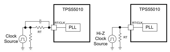
Figure 19. Synchronizing to a System Clock
