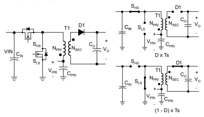
Figure 20. Output Voltage Conversion Ratio
