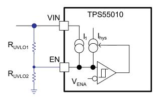
Figure 18. Adjustable Under Voltage Lock Out
