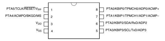
Figure 5. MC9RS08KB12 Series 8-Pin SOIC/DFN Package
