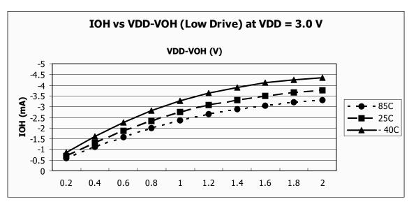
Figure 21. Typical  $I_{OH}$  vs.  $V_{DD}-V_{OH}$  $V_{DD}$  = 3 V (Low Drive)
