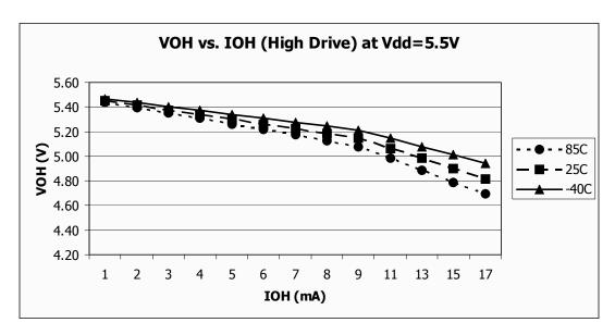
Figure 6. Typical  $V_{OH}$  vs.  $I_{OH}$  $V_{DD} = 5.5 \text{ V (High Drive)}$
