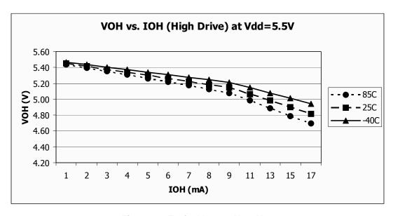
Figure 18. Typical  $I_{OH}$  vs.  $V_{DD}-V_{OH}$   $V_{DD}$  = 5.5 V (High Drive)
