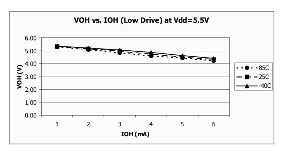
Figure 7. Typical V<sub>OH</sub> vs. I<sub>OH</sub> V<sub>DD</sub> = 5.5 V (Low Drive)
