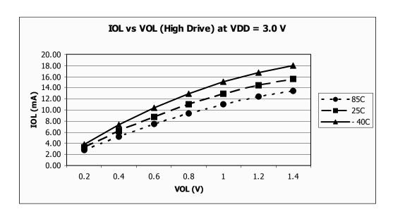
Figure 26. Typical  $I_{OL}$  vs.  $V_{OL}$  $V_{DD}$  = 3 V (High Drive)
