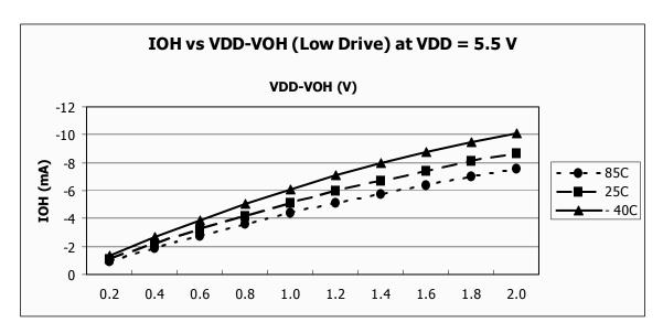
Figure 19. Typical  $I_{OH}$  vs.  $V_{DD}-V_{OH}$  $V_{DD}=5.5$  V (Low Drive)
