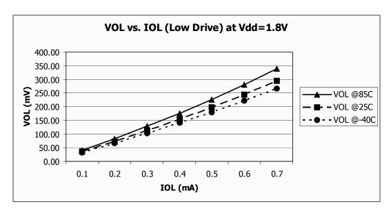
Figure 17. Typical  $V_{OL}$  vs.  $I_{OL}$   $V_{DD} = 1.8 \text{ V (Low Drive)}$
