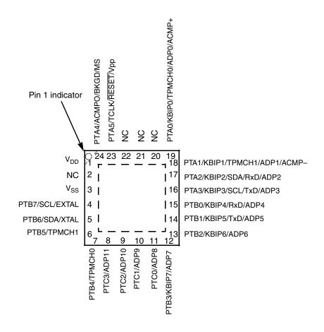
Figure 2. MC9RS08KB12 Series 24-Pin QFN Package
