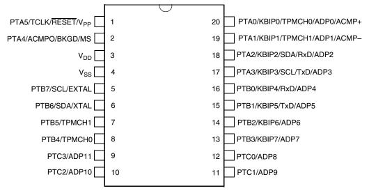
Figure 3. MC9RS08KB12 Series 20-Pin SOIC Package
