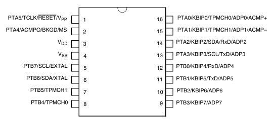
Figure 4. MC9RS08KB12 Series 16-Pin SOIC NB/TSSOP Package
