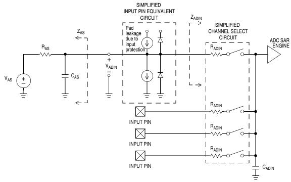
Figure 34. ADC Input Impedance Equivalency Diagram
