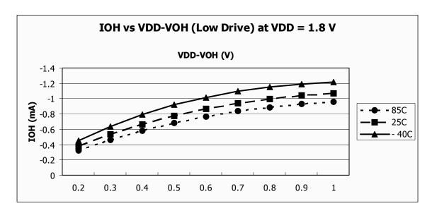
Figure 23. Typical  $I_{OH}$  vs.  $V_{DD}$ – $V_{OH}$   $V_{DD}$  = 1.8 V (Low Drive)
