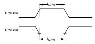
Figure 33. Timer Input Capture Pulse
