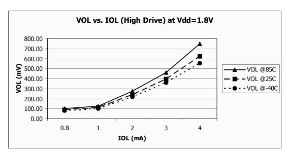
Figure 16. Typical  $V_{OL}$  vs.  $I_{OL}$   $V_{DD}$  = 1.8 V (High Drive)
