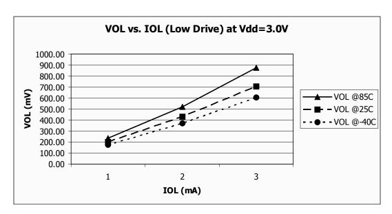
Figure 15. Typical  $V_{OL}$  vs.  $I_{OL}$   $V_{DD} = 3.0 \text{ V (Low Drive)}$
