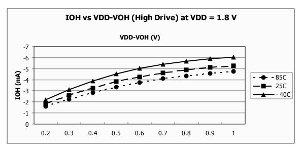
Figure 22. Typical  $I_{OH}$  vs.  $V_{DD}-V_{OH}$   $V_{DD}$  = 1.8 V (High Drive)
