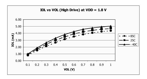
Figure 28. Typical  $I_{OL}$  vs.  $V_{OL}$   $V_{DD}$  = 1.8 V (High Drive)
