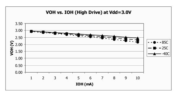
Figure 8. Typical  $V_{OH}$  vs.  $I_{OH}$   $V_{DD}$  = 3.0 V (High Drive)
