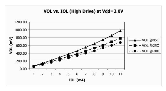
Figure 14. Typical  $V_{OL}$  vs.  $I_{OL}$   $V_{DD}$  = 3.0 V (High Drive)
