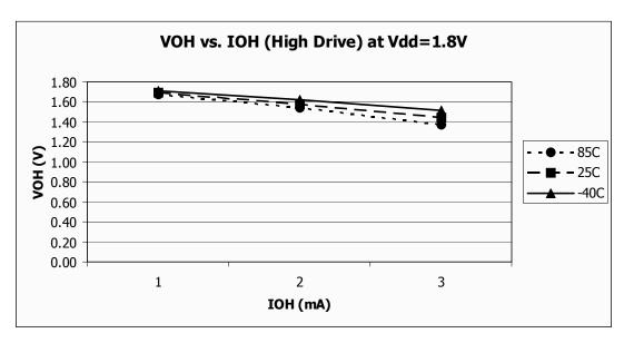
Figure 10. Typical  $V_{OH}$  vs.  $I_{OH}$   $V_{DD}$  = 1.8 V (High Drive)
