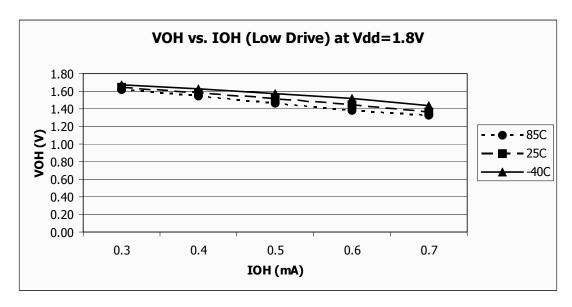
Figure 11. Typical  $V_{OH}$  vs.  $I_{OH}$   $V_{DD}$  = 1.8 V (Low Drive)
