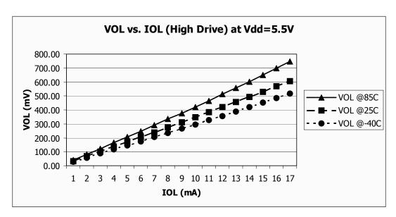
Figure 12. Typical  $V_{OL}$  vs.  $I_{OL}$   $V_{DD}$  = 5.5 V (High Drive)
