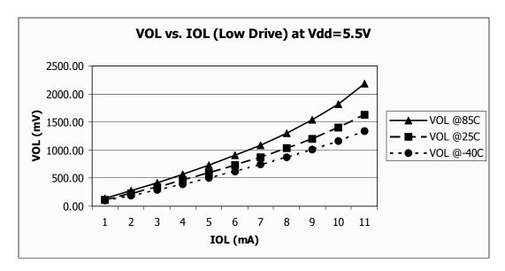
Figure 13. Typical  $V_{OL}$  vs.  $I_{OL}$  $V_{DD}$  = 5.5 V (Low Drive)
