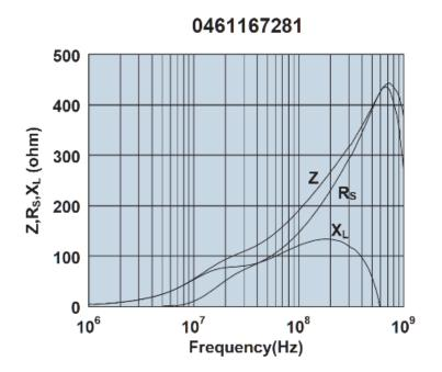
Impedance, reactance, and resistance vs. frequency.
