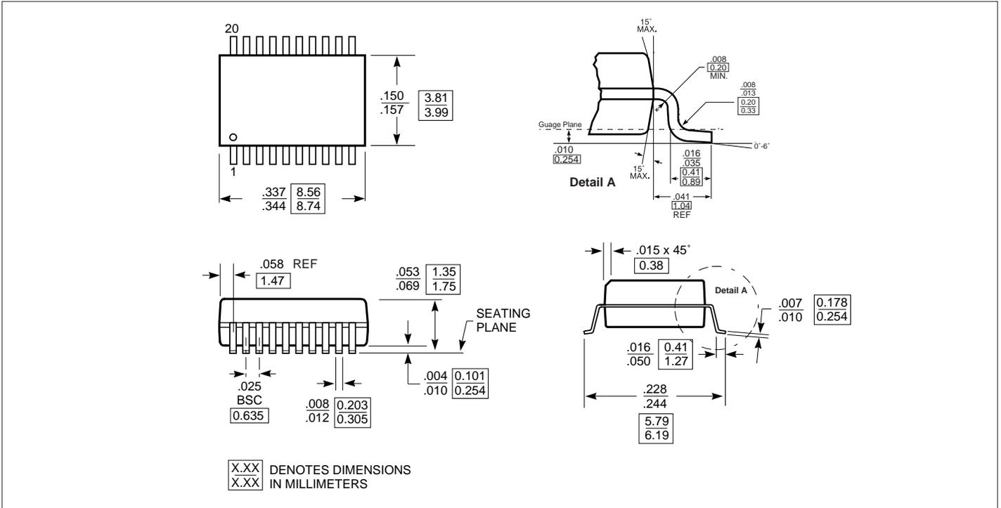
**Packaging Mechanical: 20-Pin SSOP (H)**
