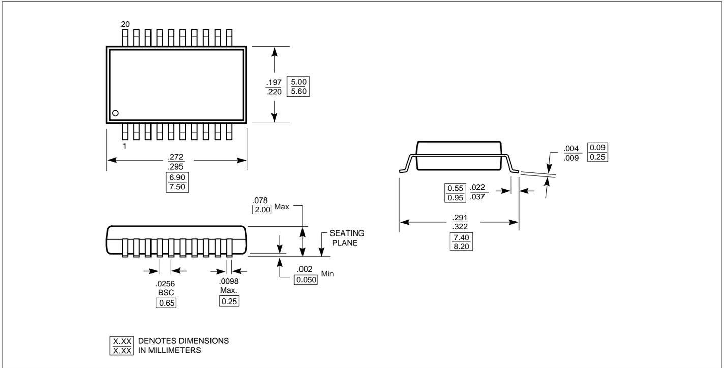
**Packaging Mechanical: 20-pin SOIC (S)**
