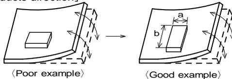
Products shall be located in the sideways direction (Length:  $a < \cdot b$ ) to the mechanical stress.
