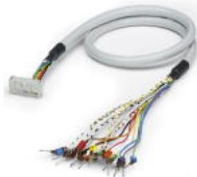
Round cable assembled with a 16-pos. socket strip and an open end. On the open end, the wires are labeled with 1 to 16 and have ferrules, cable length: 4.0 m
