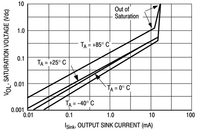
Figure 5. Output Saturation Voltage versus Output Sink Current
