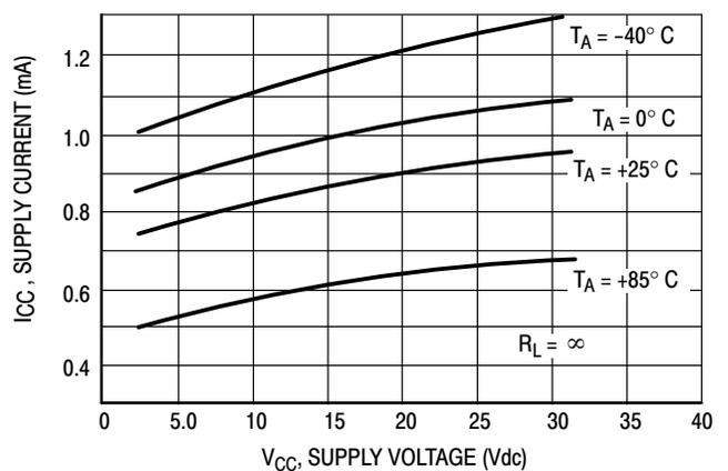
Figure 7. Power Supply Current versus Power Supply Voltage
