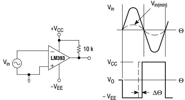
$$V_{in(min)} \approx 0.4\text{ V peak for } 1\% \text{ phase distortion } (\Delta\Theta).$$
