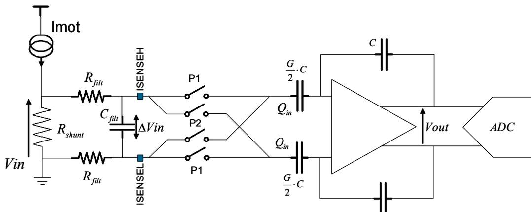
Figure 39. Current Sense Module with External Filter Option
