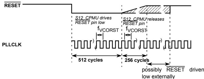
Figure 95. RESET Timing
