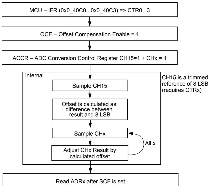
**Figure 38. Automatic Offset Compensation**
