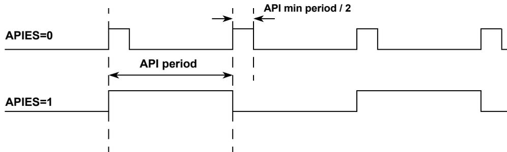
**Figure 86. Waveform selected on API\_EXTCLK pin (APIEA=1, APIFE=1)**
