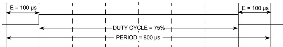
Figure 30. PWM Center Aligned Output Example Waveform
