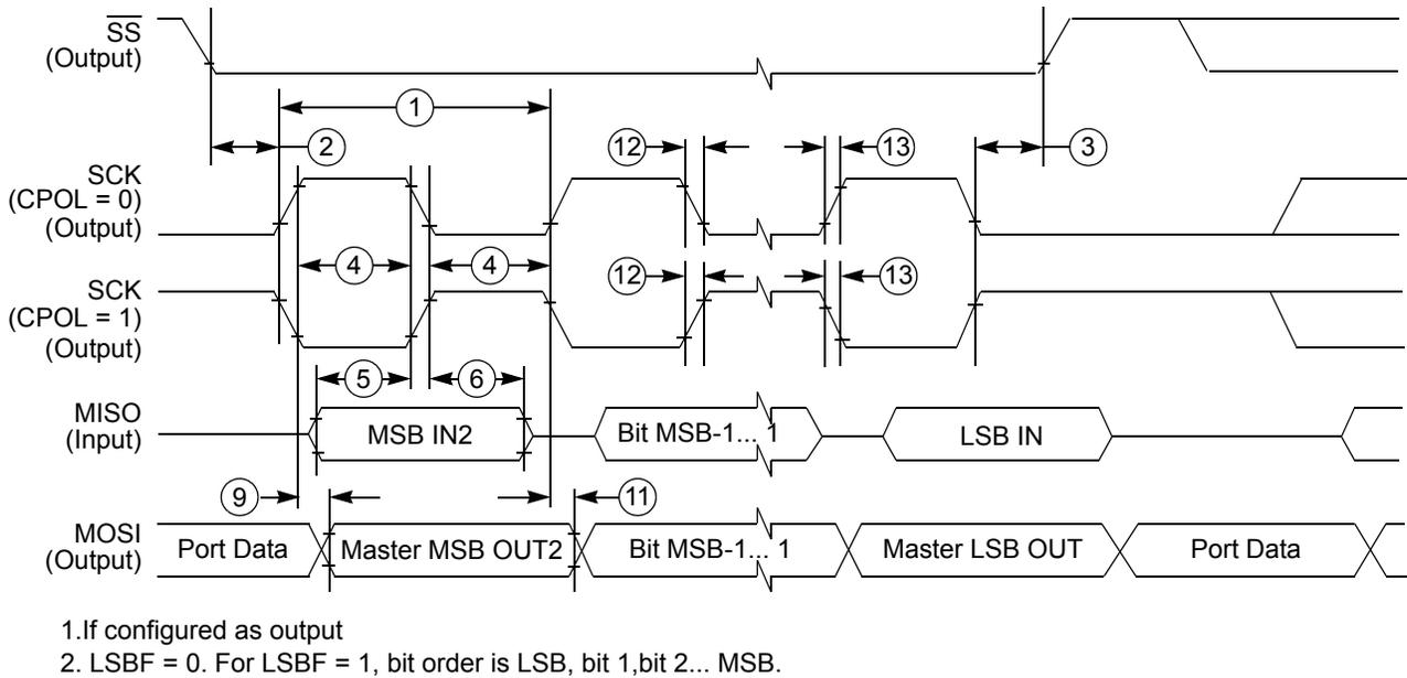
**Figure 13. SPI Master Timing (CPHA = 1)**
