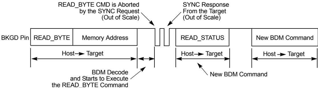
**Figure 62. ACK Abort Procedure at the Command Level**
