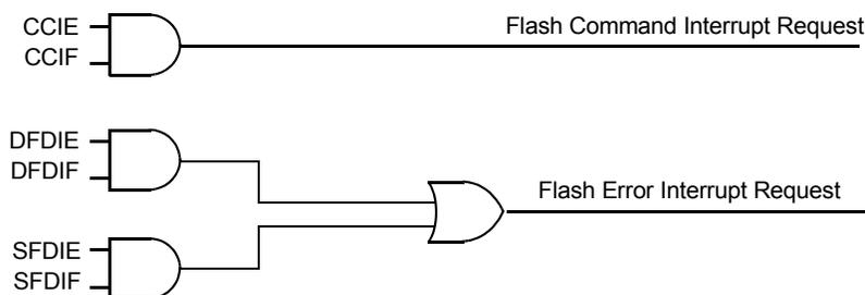
**Figure 110. Flash Module Interrupts Implementation**
