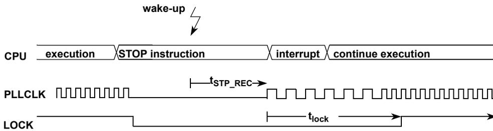
Figure 90. Stop Mode Using PLLCLK as Bus Clock
