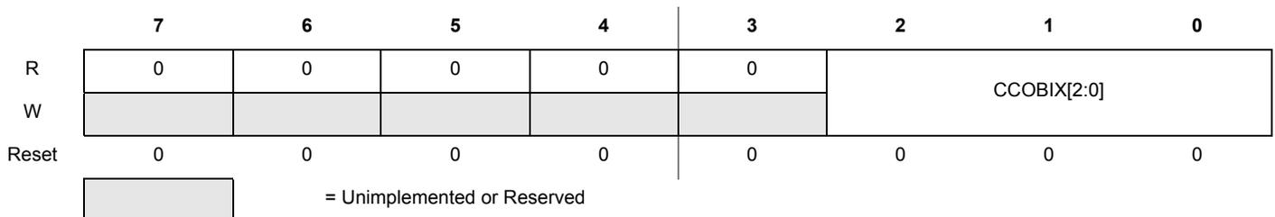
CCOBIX bits are readable and writable while remaining bits read 0 and are not writable.
