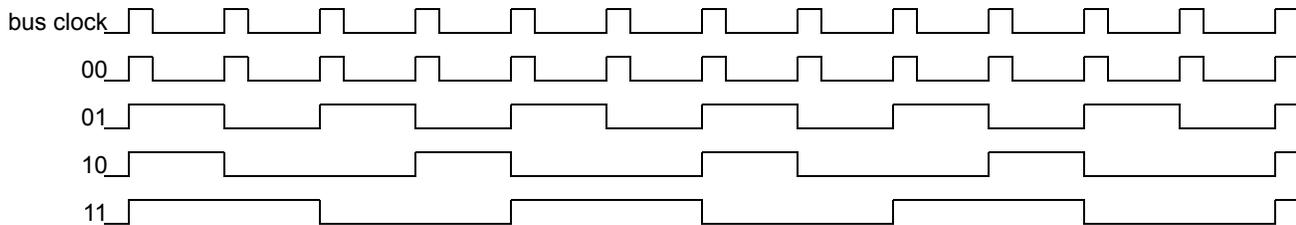
**Figure 113. Interface Clock Waveforms for various D2DCLKDIV Encoding**
