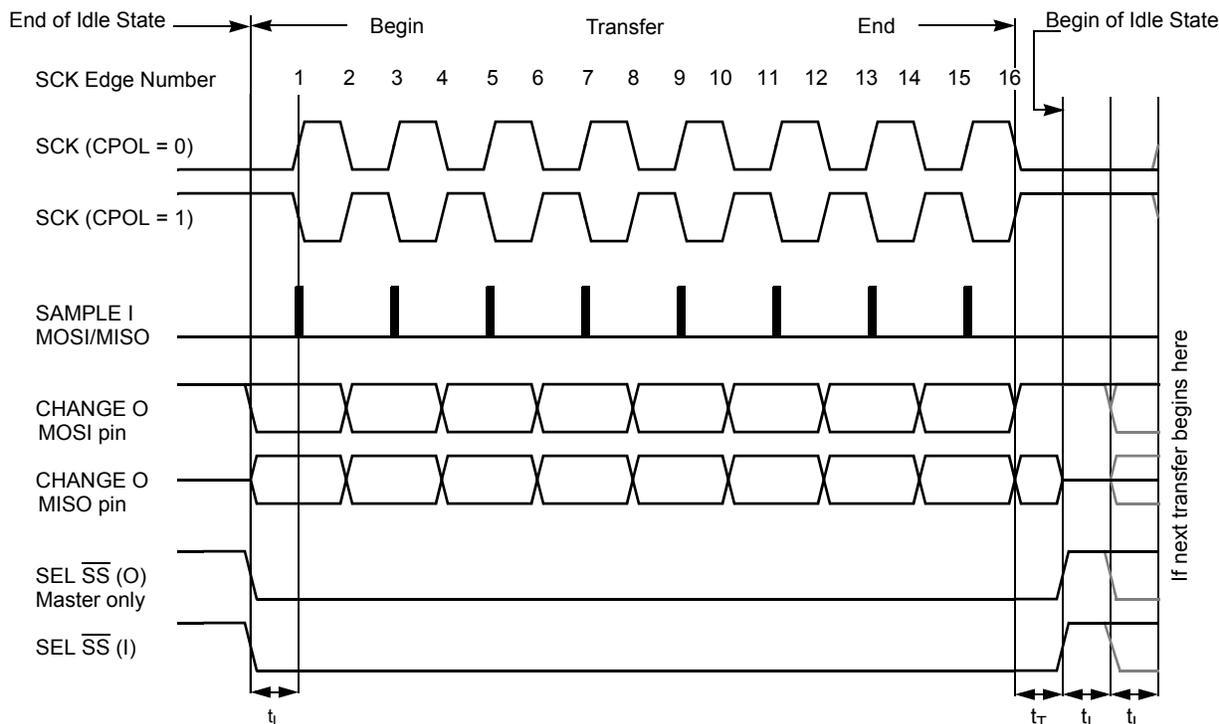
MSB first (LSBFE = 0): MSB Bit 6 Bit 5 Bit 4 Bit 3 Bit 2 Bit 1 LSB Minimum 1/2 SCK
