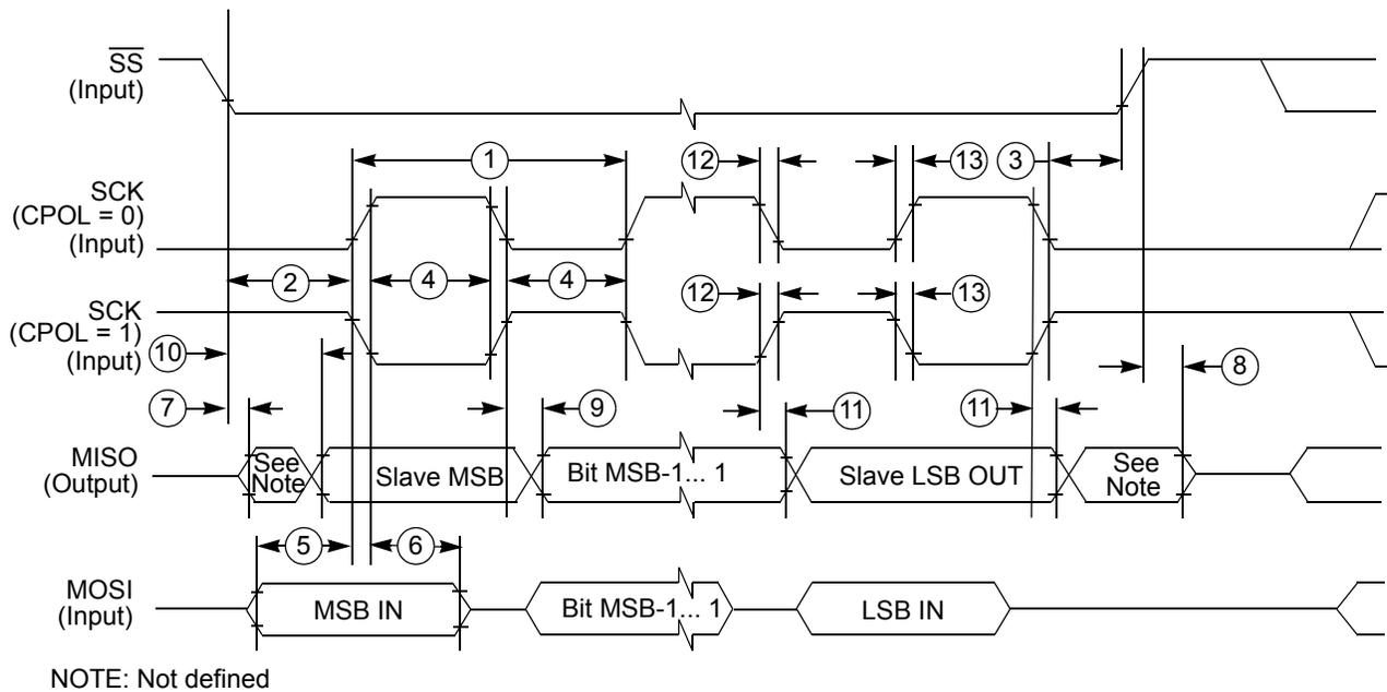
**Figure 14. SPI Slave Timing (CPHA = 0)**
