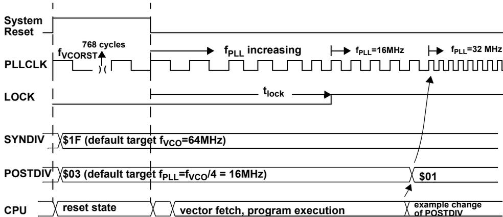
Figure 89. Startup of Clock System After Reset
