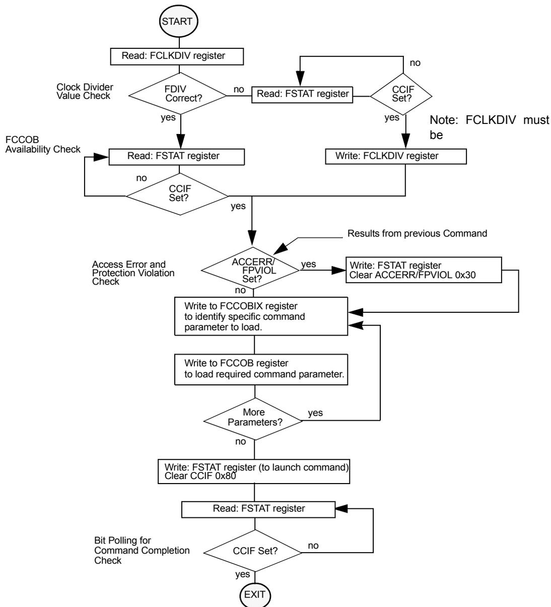
Figure 109. Generic Flash Command Write Sequence Flowchart
