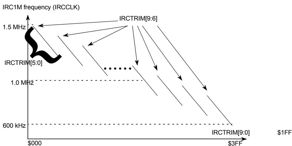
**Figure 87. IRC1M Frequency Trimming Diagram**
