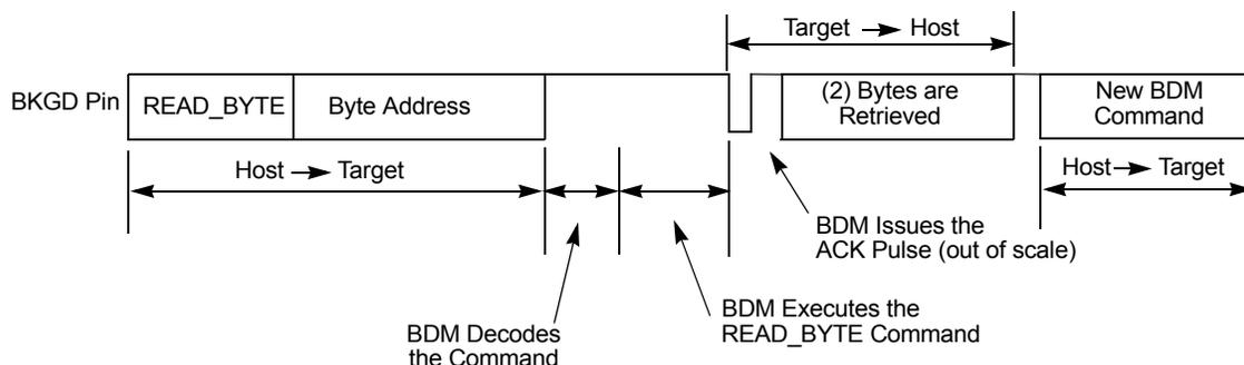
Figure 61. Handshake Protocol at the Command Level
