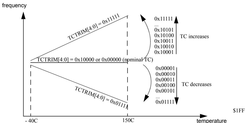
**Figure 88. Influence of TCTRIM[4:0] on the Temperature Coefficient**
