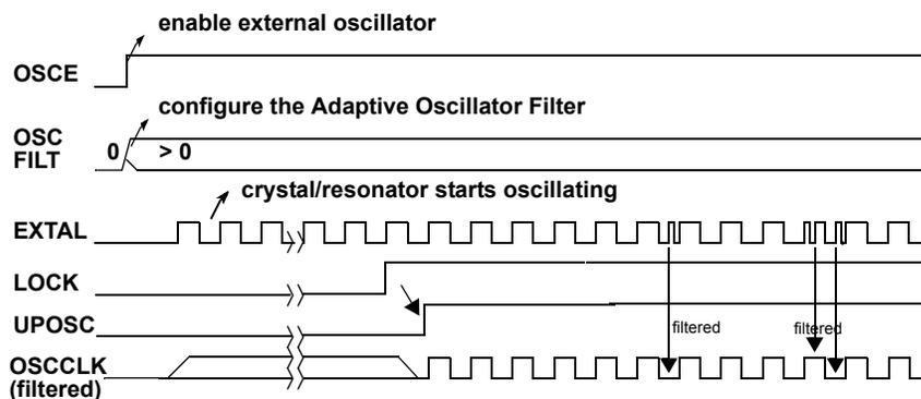
**Figure 93. Noise Filtered by the Adaptive Oscillator Filter**
