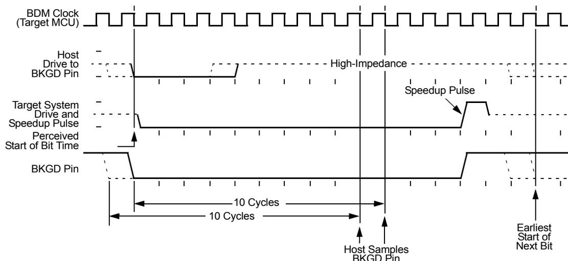
**Figure 59. BDM Target-to-Host Serial Bit Timing (Logic 0)**
