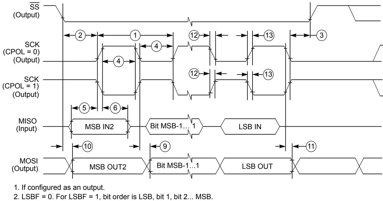
**Figure 12. SPI Master Timing (CPHA = 0)**
