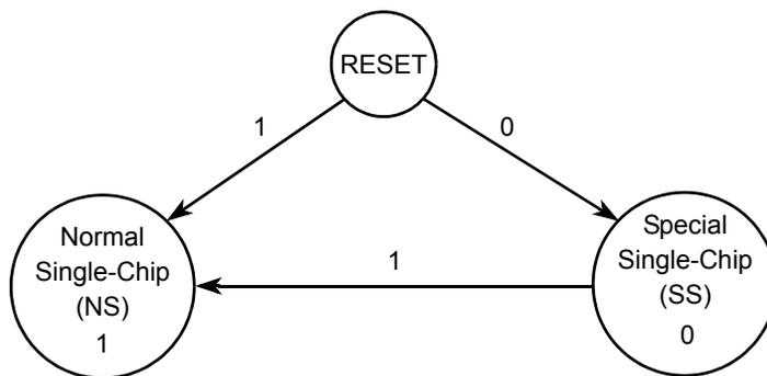
**Figure 47. Mode Transition Diagram When MCU is Unsecured**
