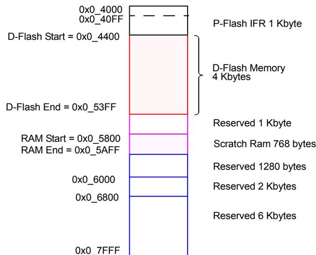
**Figure 107. D-Flash and Memory Controller Resource Memory Map**
