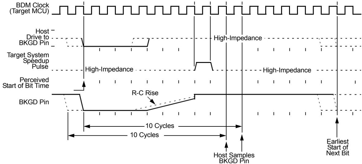
**Figure 58. BDM Target-to-Host Serial Bit Timing (Logic 1)**
