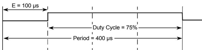
Figure 28. PWM Left Aligned Output Example Waveform
