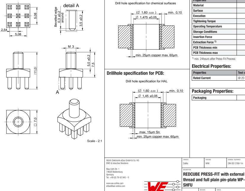
**Drillhole specification for PCB:**
