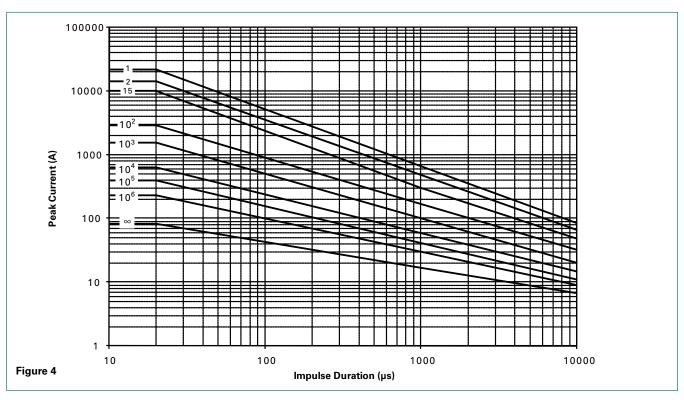
**Note:** Repetitive surge capability is qualified and tested based on 8/20us current waveform (not combination waveform) and UL1449 40.7.3 (Edition 4) test condition.
