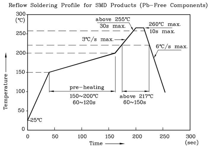
1. All temperatures refer to the center of the package, measured on the package body surface facing up during reflow.
