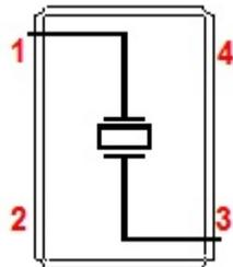
Pad 2 and Pad 4 are common and connected to the metal cover. They are not connected to the crystal. Connected to ground is recommended
