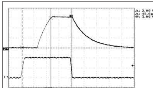
Turn-on Characteristic ( V_{IN} = 4V , I_{OUT}=100mA )
