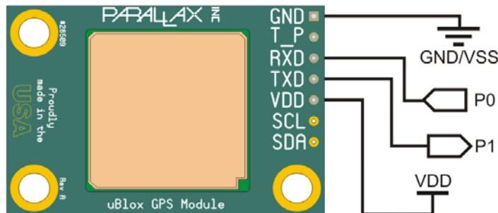
The PAM-7Q GPS Module can be interfaced with many common microcontrollers or computers, including the Propeller, BASIC Stamp, Arduino, PIC, Raspberry Pi, Beaglebone, and more. At minimum, you can begin receiving data from the module by connecting the power pins, VDD and GND, and by making a connection with the module's transmit pin, TXD. If you want to change any of the module's settings, you will need to connect a signaling pin from your device to the module's receive pin, RXD.
