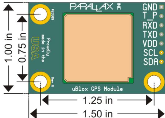
Pin spacing is standard 0.1" for a breadboard friendly design. Mounting holes are spaced by 1.25" and 0.75" center-to-center, with a .125" diameter, and accepts #4-40 screws.
