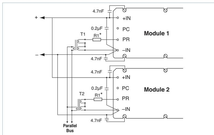
Figure 10 — Transformer-coupled interface
