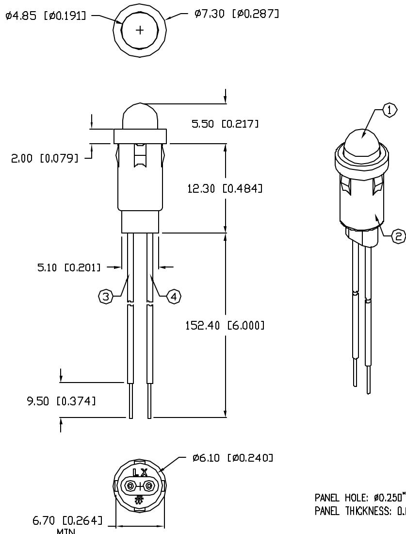
\*UNLESS OTHERWISE SPECIFIED TOLERANCES PER DECIMAL PRECISION ARE: X=±1 (±0.039), XX=±0.5 (±0.020), XXX=±0.25 (±0.010), XXXX=±0.127 (±0.005). LEAD SIZE=±0.05 (±0.002), LEAD LENGTH=±0.75 (±0.030). MIN= <sup>+0.00</sup><sub>-0.00</sub> DECIMAL PRECISION MAX= <sup>+0.00</sup><sub>-0.00</sub> DECIMAL PRECISION
