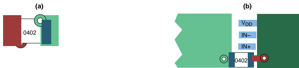
Figure 18. Typical Decoupling Capacitor Layouts
