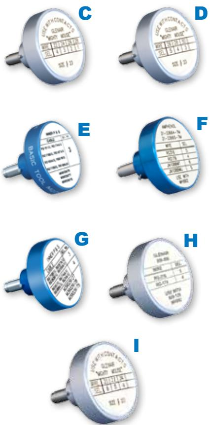
These bayonet-type positioners hold contacts at correct height for crimping with M22520/2 type miniature step adjustable tools, above. Face plate shows correct tool settings.
