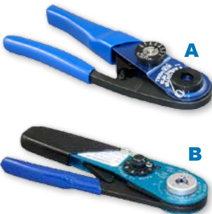
These crimp tools perform precision eight indent crimps for gas tight wire terminations and excellent tensile strength. Adjustment wheel has 8 settings. Ratchet mechanism prevents improper crimps. Use with bayonet type positioners. Check calibration with M22520/3 gages. Length is 6.75 inches, weight is approx. 10 oz.
