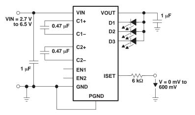
Figure 13. Analog Dimming Connections Using ISET Pin
