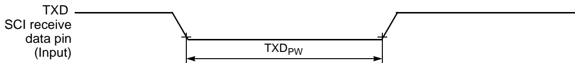
Figure 10-17 TXD Pulse Width
