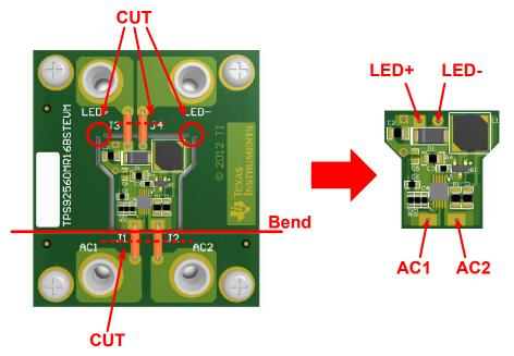
Figure 3. Removing Outer Frame of the TPS92560MR16BSTEVM
