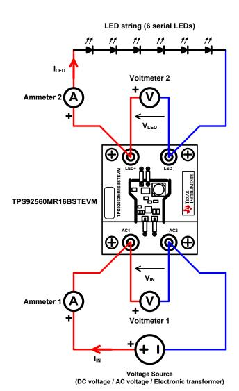
Figure 4. Connection Diagram of the TPS92560MR16BSTEVM
