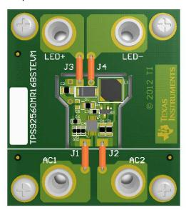
Figure 2. TPS92560MR16BSTEVM Input and Output Terminals
