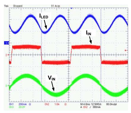
6 serial LEDs,  $T_A = 25^{\circ}C$  $I_{LED}$ : 200 mA/DIV,  $I_{IN}$ : 1 A/DIV,  $V_{IN}$ : 20 V/DIV
