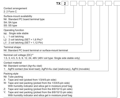
Note 1) In case of 5 V transistor drive circuit, it is recommended to use 4.5 V type relay Note 2) Please contact our sales representative for detailed specifications.
