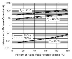
Fig. 4 - Typical Reverse Characteristics
