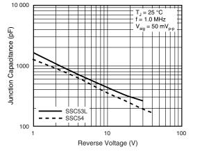
Fig. 5 - Typical Junction Capacitance
