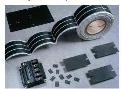
Q-Pad® 3 eliminates problems associated with thermal grease such as contamination of electronic assemblies and reflow solder baths. Q-Pad® 3 may be installed prior to soldering and cleaning without worry. When clamped between two surfaces, the elastomer conforms to surface textures thereby creating an air-free interface between heat-generating components and heat sinks.
