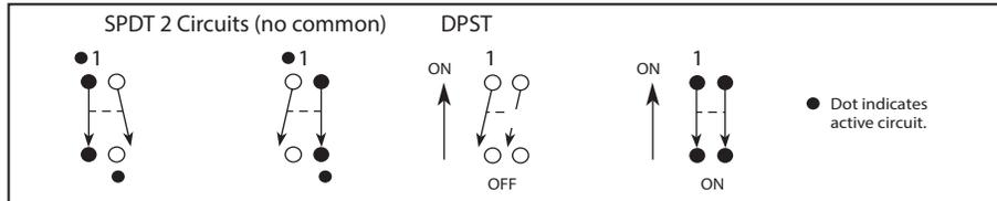
with all actuators in the closed (on) position as shipped.
