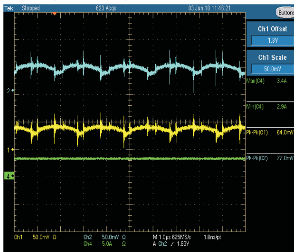
Figure 10. Ripple for Buck 1 (Yellow Trace) 1.2 V, 3 A and Buck 2 (Blue Trace) 1.8 V, 2 A, 50 mV per Division V_{IN} = 12\text{ V} , f_{SW} = 500\text{ kHz} , L_O = 4.7\text{ }\mu\text{H} , DCR = 10\text{ m}\Omega , C_O = 22\text{ }\mu\text{F}
