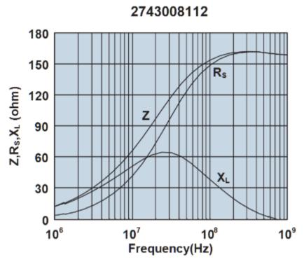
Impedance, reactance, and resistance vs. frequency.
