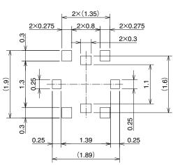
: This area must be free of conductive traces and solder resist on top layer.
