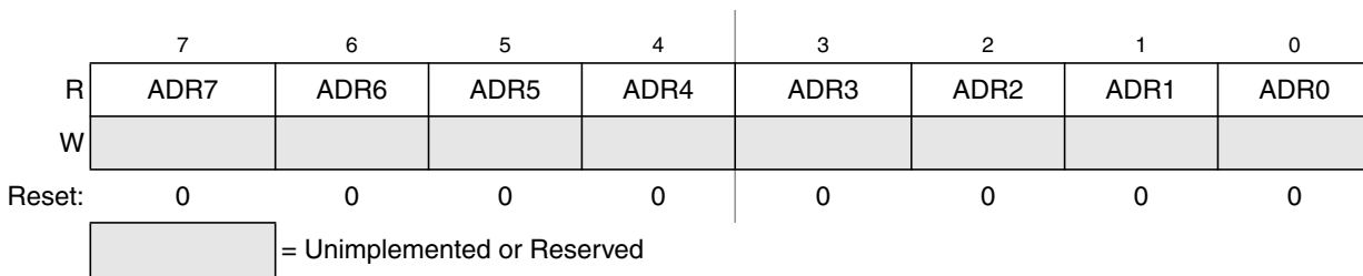
Figure 14-7. Data Result Low Register (ADC1RL)
