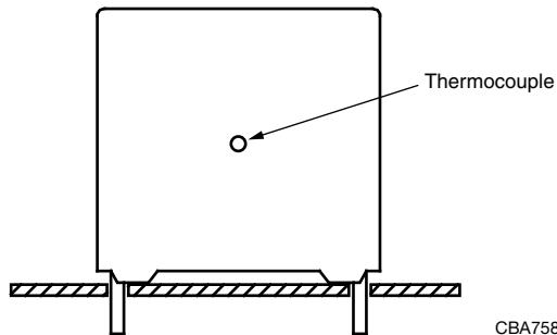
The temperature is measured in unloaded ( $T_{\text{amb}}$ ) and maximum loaded condition ( $T_C$ ).
