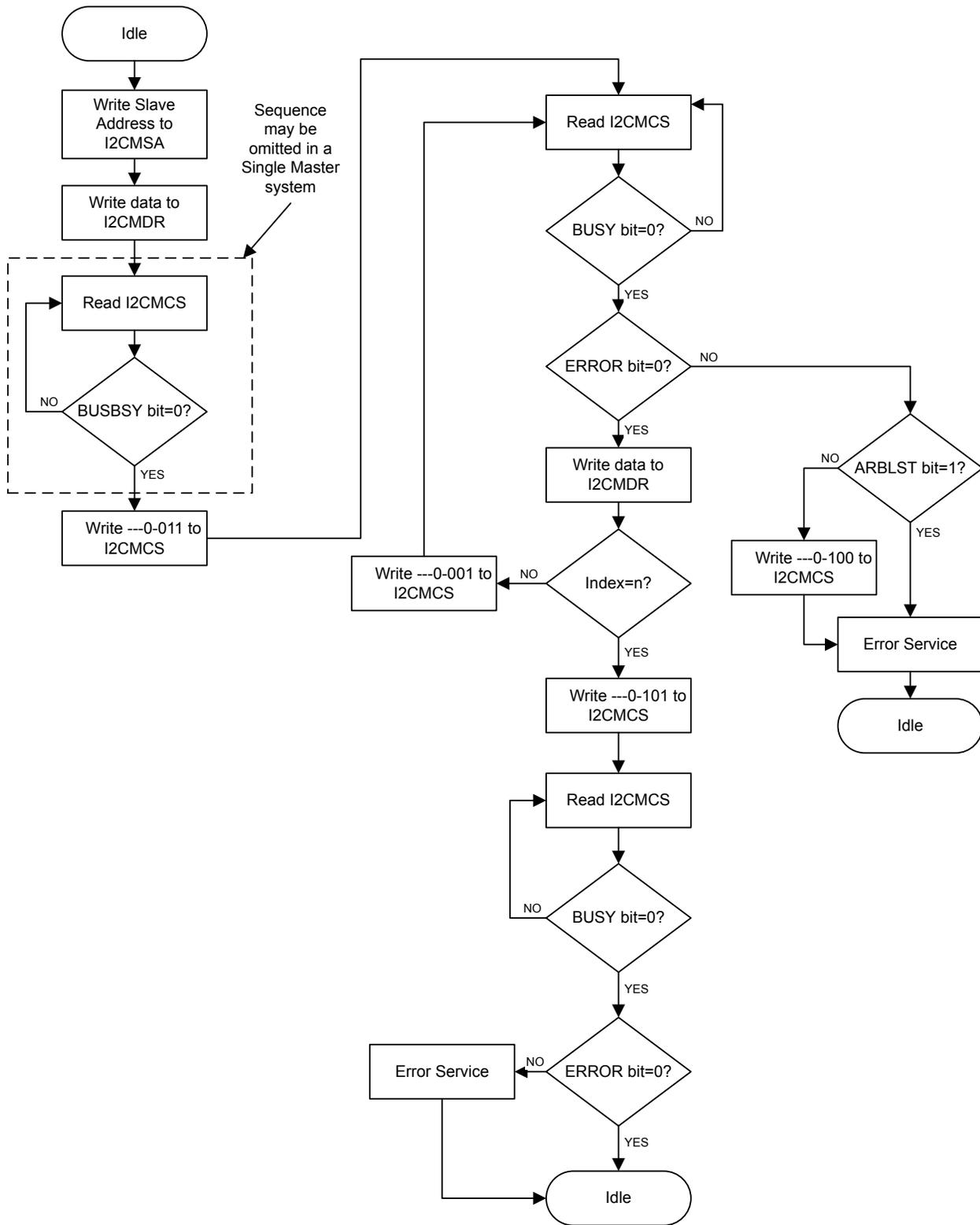
Figure 13-10. Master Burst RECEIVE
