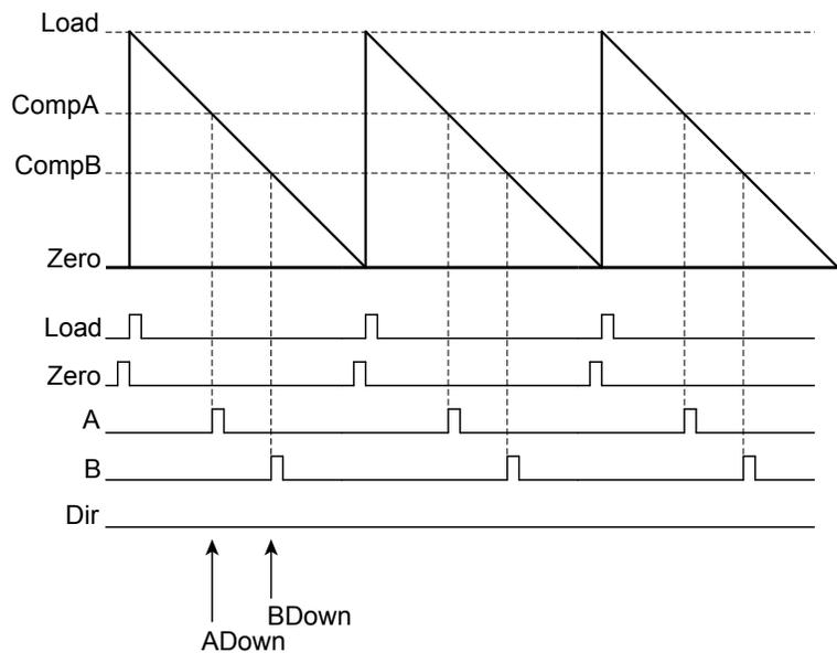
**Figure 15-4. PWM Count-Up/Down Mode**
