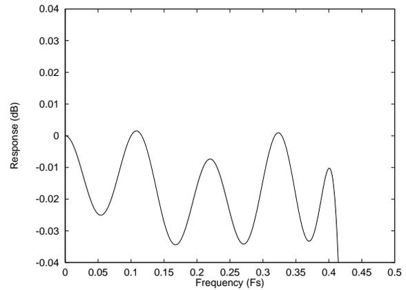
Figure 36 DAC Digital Filter Ripple –Type 0
