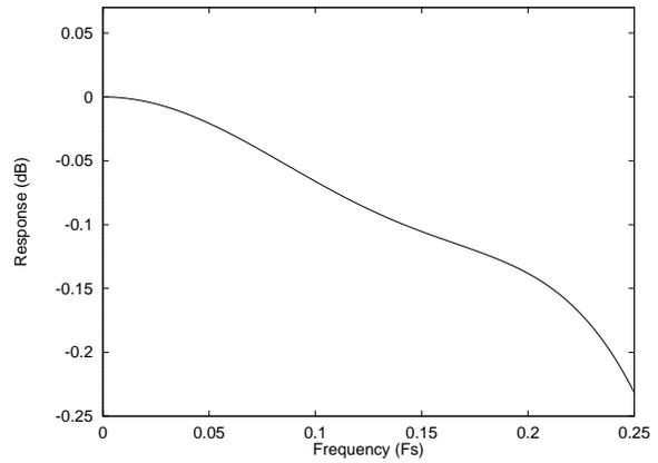
Figure 42 DAC Digital Filter Ripple –Type 3
