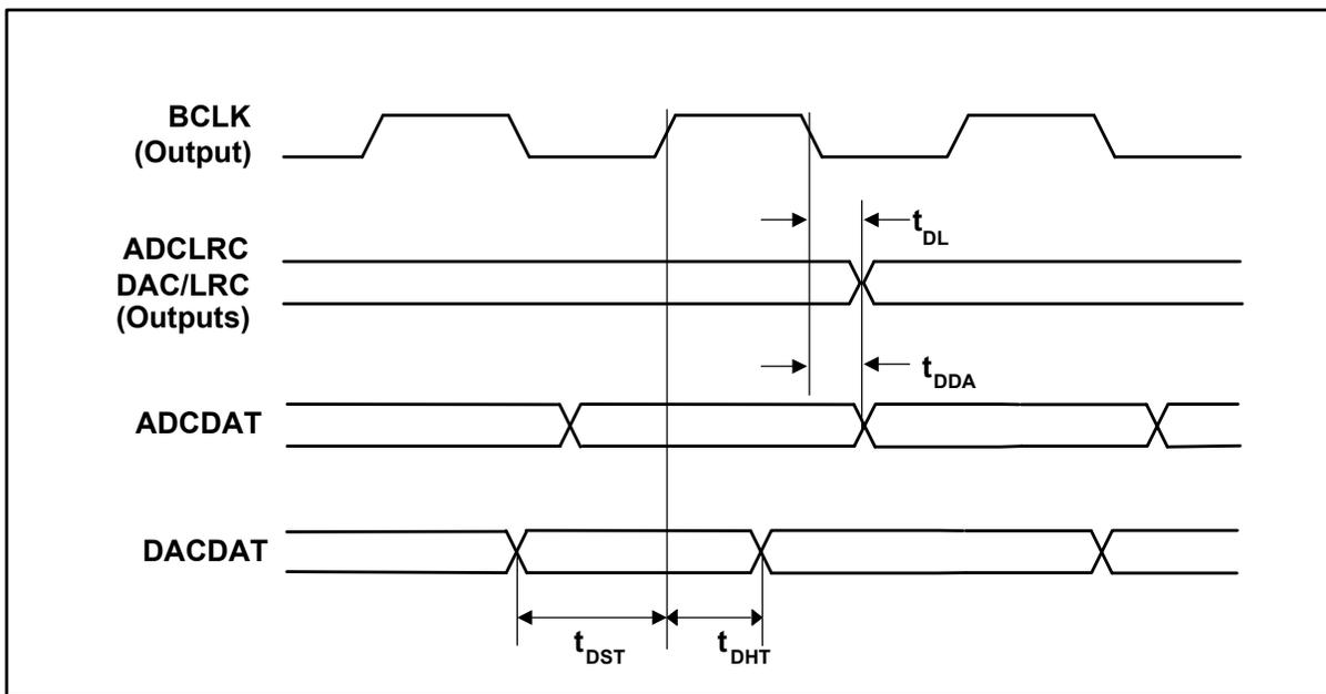
Figure 4 Digital Audio Data Timing – Master Mode
