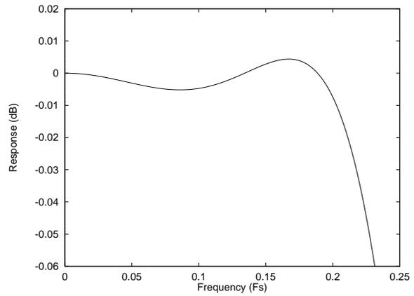
Figure 48 ADC Digital Filter Ripple –Type 2
