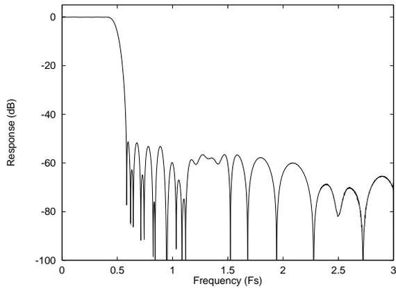
Figure 35 DAC Digital Filter Frequency Response –Type 0
