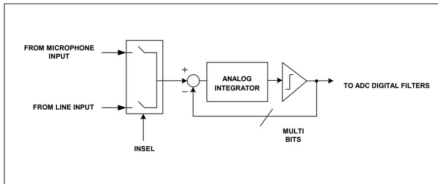
Figure 15 Multi-Bit Oversampling Sigma Delta ADC Schematic
