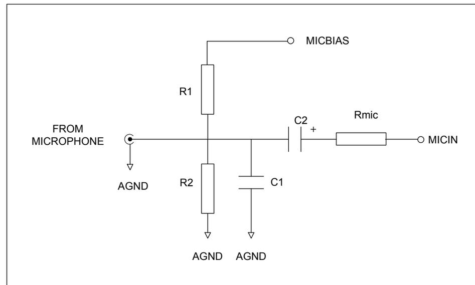
**Figure 13 Microphone Input and Bias Application Drawing**
