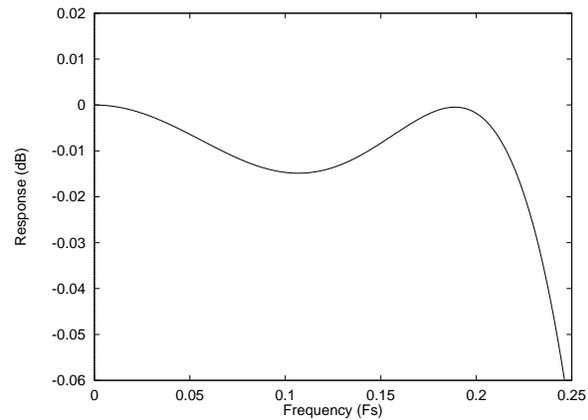
Figure 40 DAC Digital Filter Ripple –Type 2
