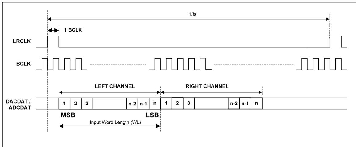
Figure 29 DSP/PCM Mode Audio Interface (mode A, LRP=1)
