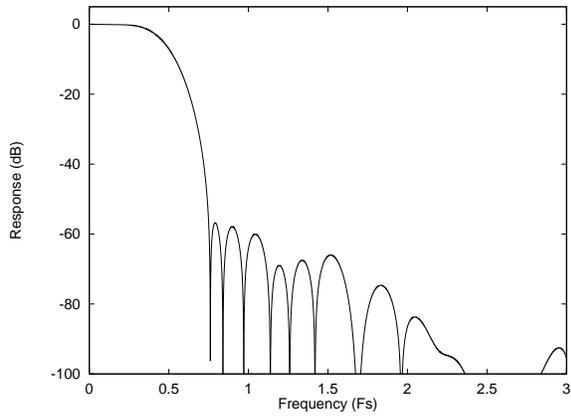
Figure 41 DAC Digital Filter Frequency Response –Type 3
