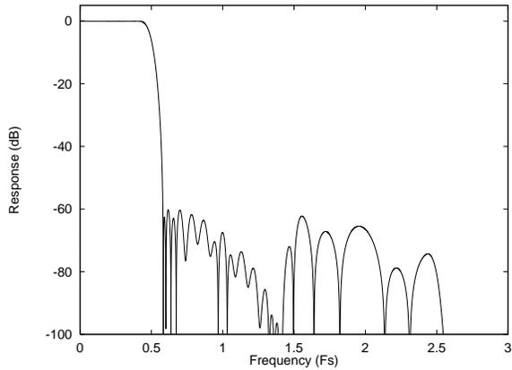
Figure 43 ADC Digital Filter Frequency Response –Type 0
