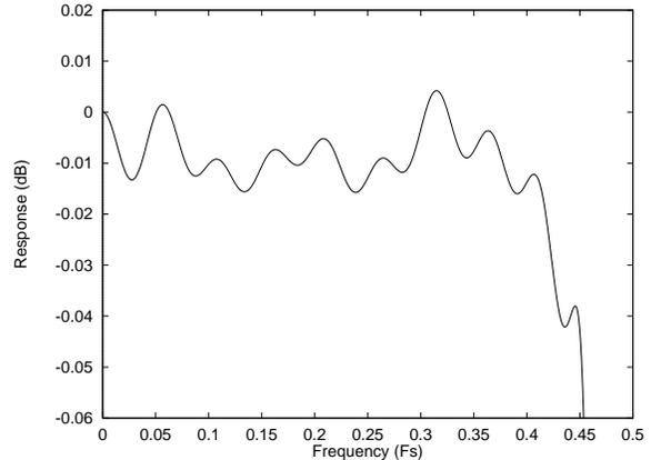
Figure 46 ADC Digital Filter Ripple –Type 1
