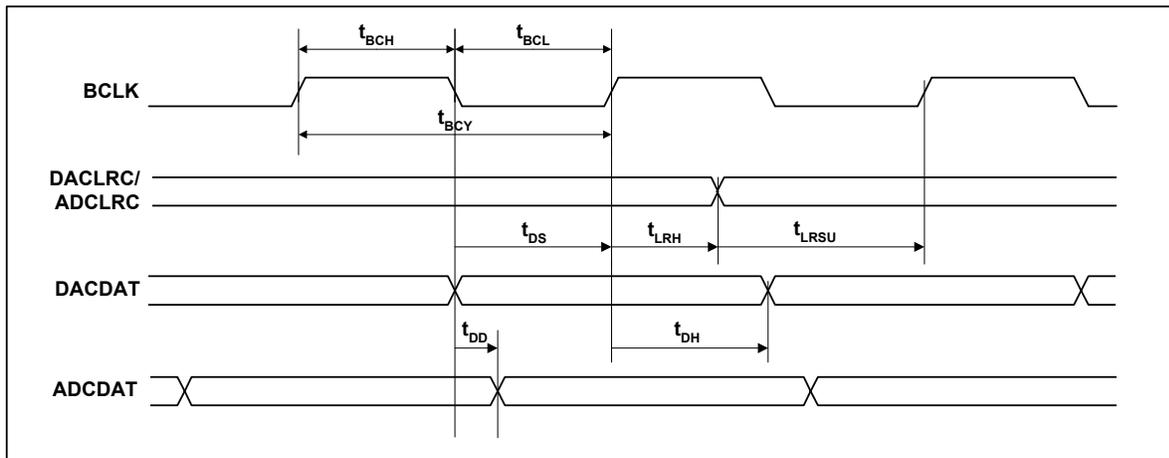
Figure 6 Digital Audio Data Timing – Slave Mode
