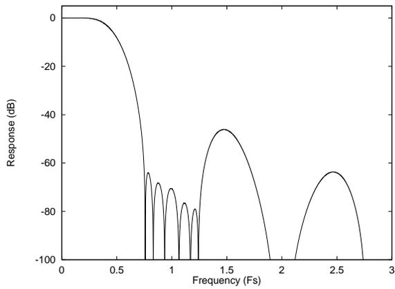
Figure 47 ADC Digital Filter Frequency Response –Type 2
