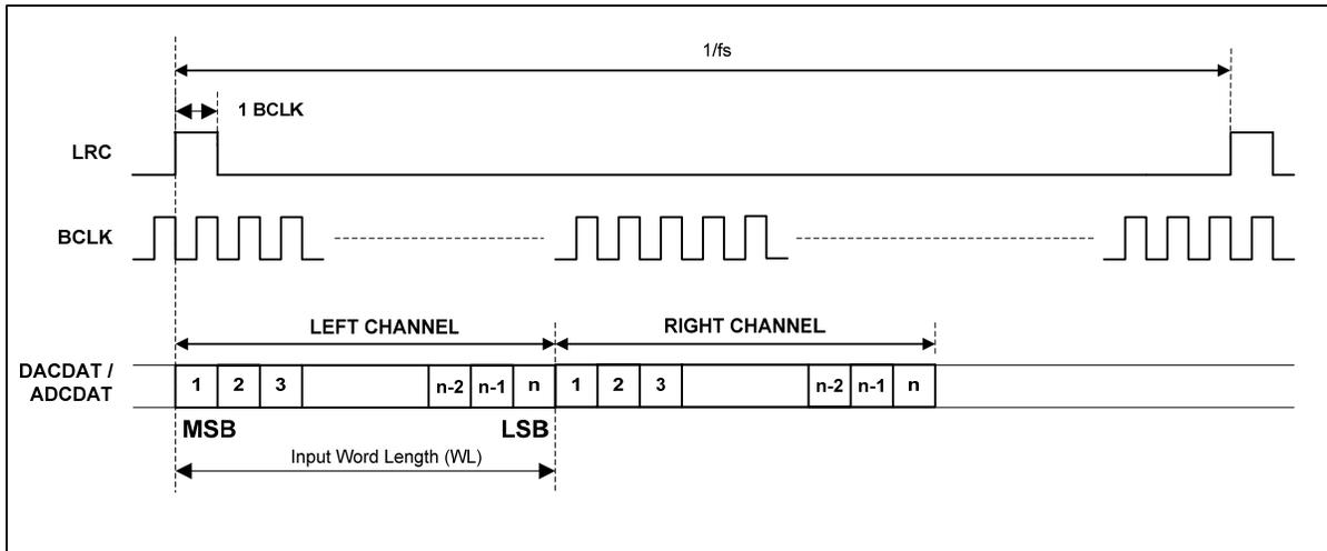
Figure 30 DSP/PCM Mode Audio Interface (mode B, LRP=0)
