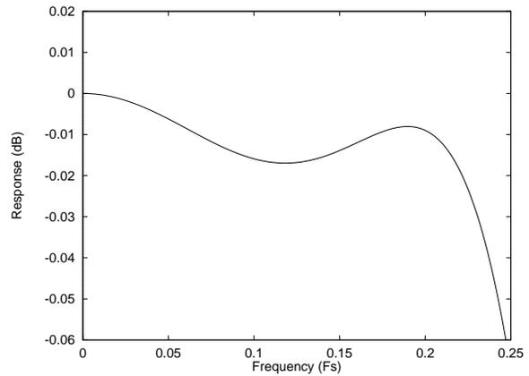
Figure 50 ADC Digital Filter Ripple –Type 3
