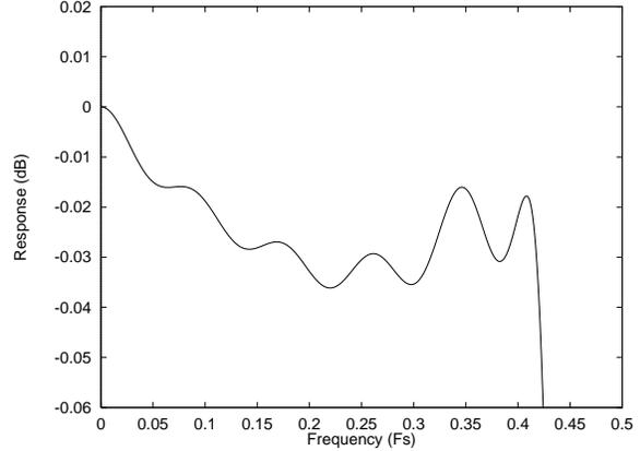
Figure 44 ADC Digital Filter Ripple –Type 0
