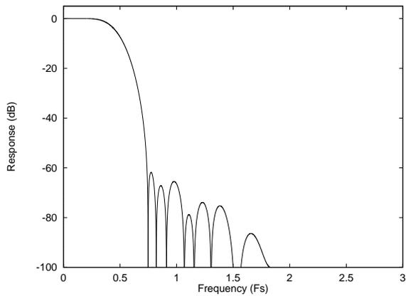
Figure 49 ADC Digital Filter Frequency Response –Type 3
