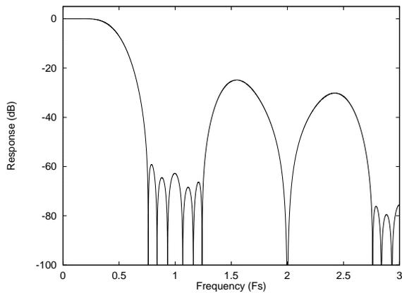
Figure 39 DAC Digital Filter Frequency Response –Type 2
