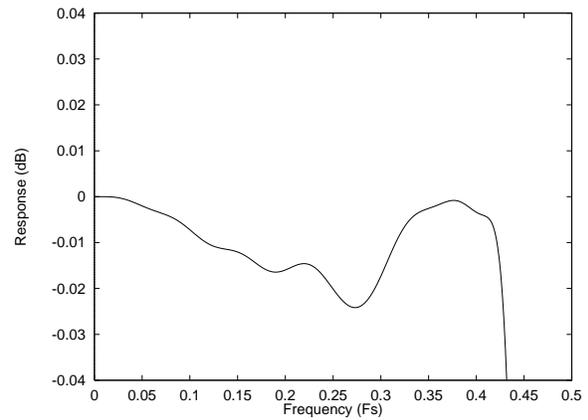
Figure 38 DAC Digital Filter Ripple –Type 1
