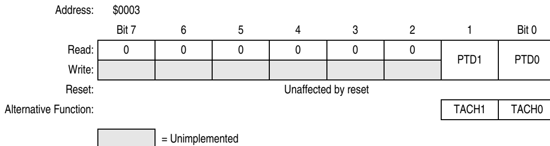
Figure 12-10. Port D Data Register (PTD)
