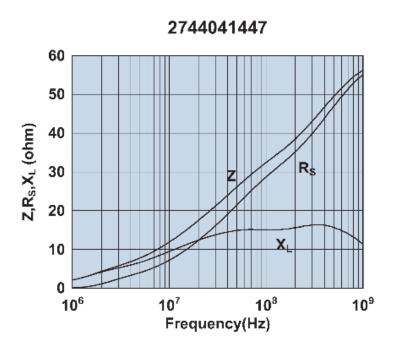
Impedance, reactance, and resistance vs. frequency.
