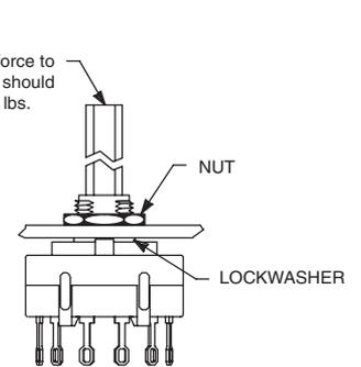
Install switch with stop ring (if used) and lockwasher in back of panel. Tighten hex nut from front of panel.
