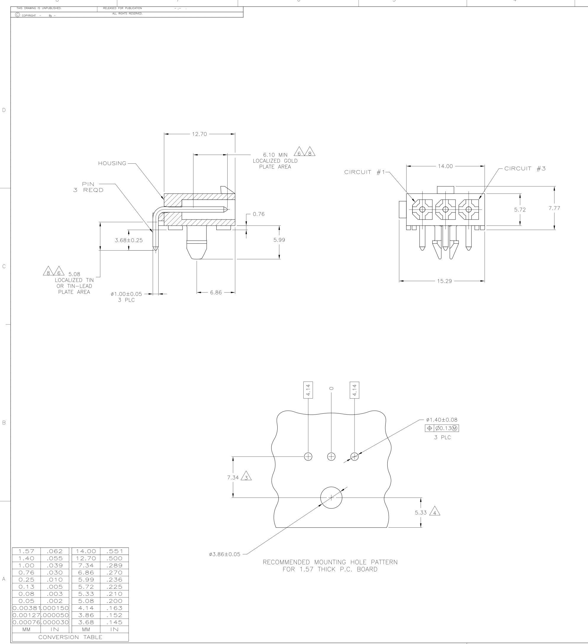
1. PINS TO COMPLY WITH AMP SOLDERABILITY SPEC 109-11-3.
