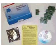
This kit supports active filters designed by FilterLab® V2.0. These filters are all pole and are built by cascading first and second order sections. The kit includes: one PCB designed to provide mid-supply biasing to the other printed circuit boards, four PCBs that support active filter designs with filter order between n = 1 and 8 (output test point for lab equipment provided) and op amps, zero ohm jumpers, resistors and capacitors that can be used to help build filters.
