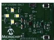
The MCP1252 board demonstrates the use of a charge pump device in an LED application and acts as a platform to evaluate the MCP1252 device in general. Light intensity is controlled uniformly through the use of ballast resistors. A PIC10F206 MCU provides an enable signal to the MCP1252 and accepts a push-button input that allows the white LEDs to be adjusted to five different light intensities.
