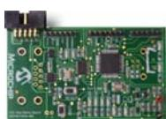
The MCP2515 CAN Bus Monitor Demo board kit contains two identical boards which can be connected together to create a simple two node Controller Area Network (CAN) bus, which can be controlled and/or monitored via the included PC interface. The board(s) can also be connected to an existing CAN bus.
