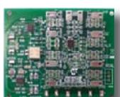
The MCP651 Input Offset Evaluation board is intended to provide a simple means to measure the MCP651 Input Offset Evaluation Board op amp's input offset voltage under a variety of operating conditions. The measured input offset voltage (VOST) includes the input offset voltage specified in the data sheet (VOS) plus changes due to: power supply voltage (PSRR), common mode voltage (CMRR), output voltage (AOL), input offset voltage drift over temperature ( $\Delta$ VOS/ $\Delta$ T) and 1/f noise.
