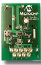
The MCP1640 Synchronous Boost Converter Evaluation board demonstrates the MCP1640 in two boost-converter applications with multiple output voltages. It can be used to evaluate both package options (SOT-23-6 and 2x3-8 DFN). This board was developed to help engineers reduce the product design cycle time.
