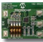
The MCP73871 Demo Board with Voltage Proportional Current Control is designed to demonstrate Microchip's stand-alone linear Li-Ion battery charger with system power path and load sharing management control solution. The MCP73871 integrates the required elements to meet design challenges when developing new Li-Ion/Li-Polymer battery powered products.
