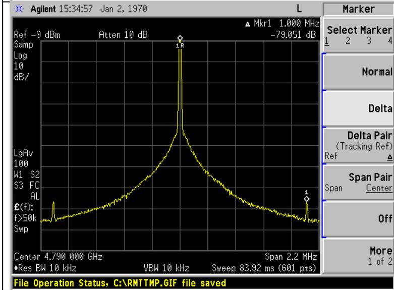
Spur at 4790 MHz VCO frequency is -79.1 dBc.
