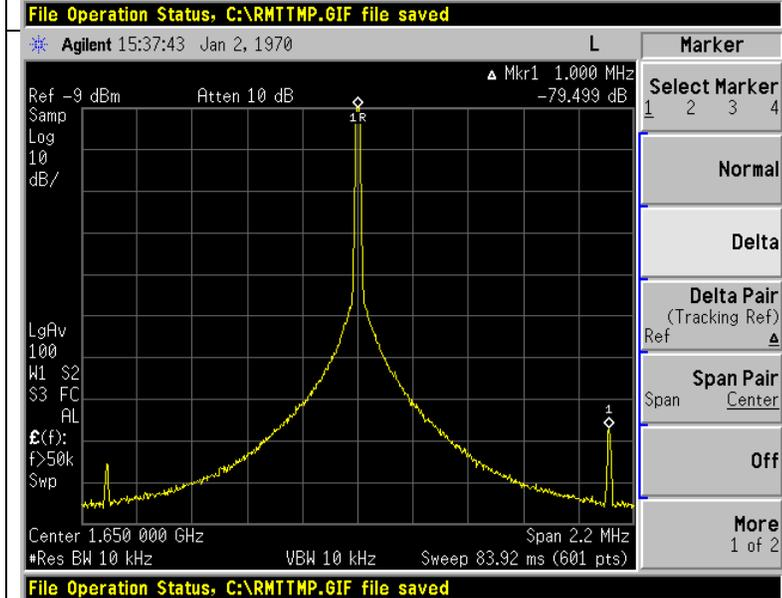
Spur at 1650 MHz VCO frequency is -79.5 dBc. Note that this spur is not symmetrical.
