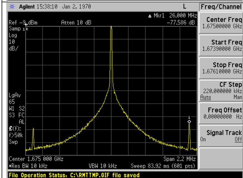
Spur at 1675 MHz VCO frequency is -77.6 dBc.
