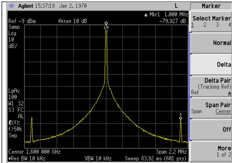
Spur at 1600 MHz VCO frequency is -79.9 dBc.
