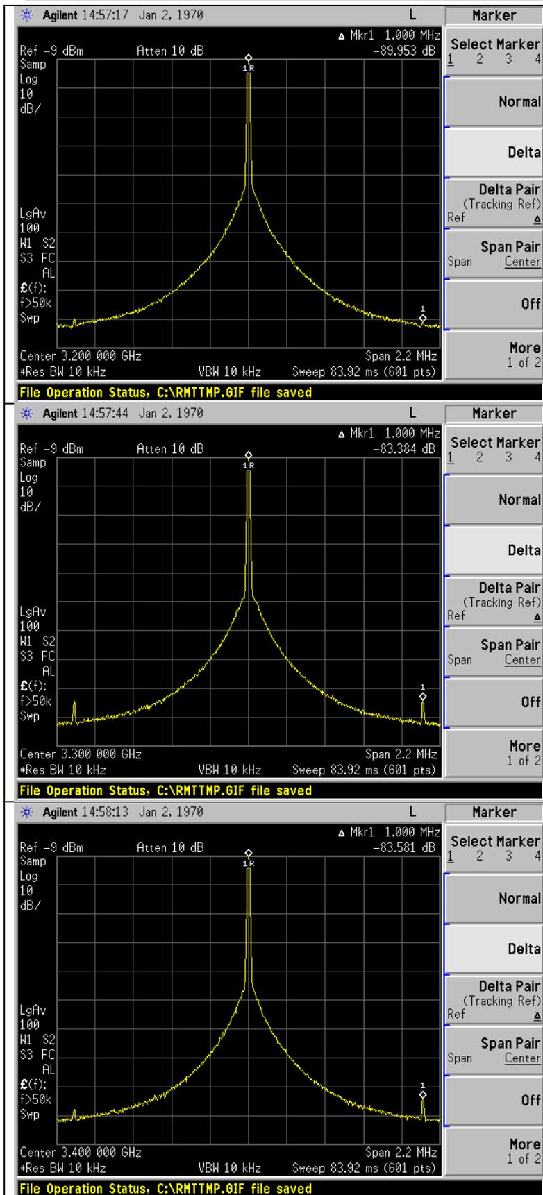
Spur at 3200 MHz VCO frequency is below the noise floor.
