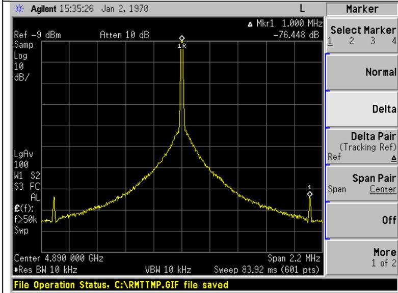
Spur at 4890 MHz VCO frequency is -76.5 dBc.
