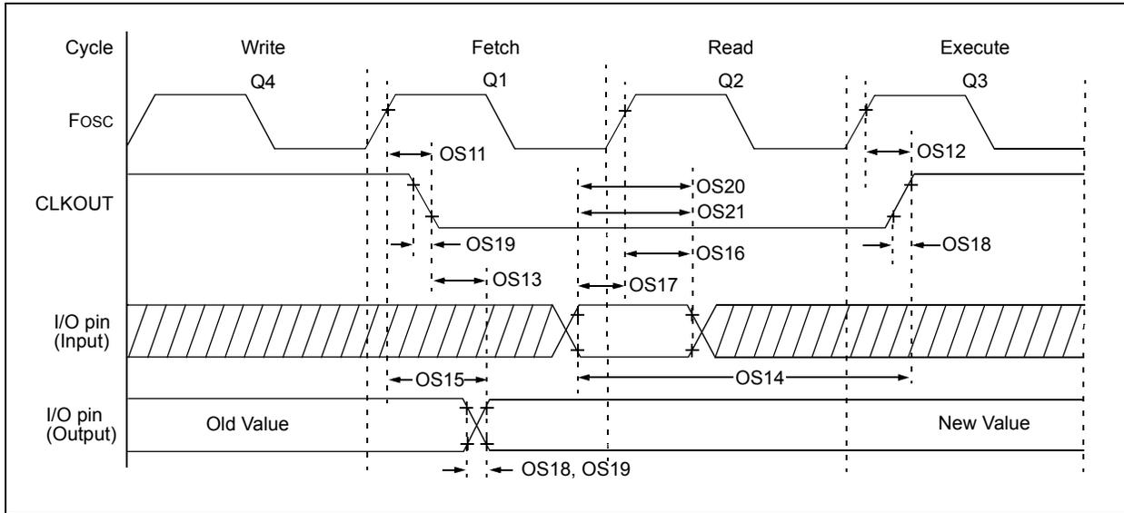
**TABLE 26-10: CLKOUT AND I/O TIMING PARAMETERS**
