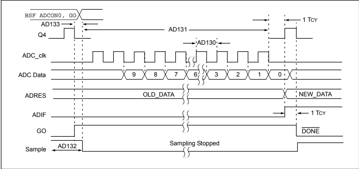
FIGURE 26-12: ADC CONVERSION TIMING (ADC CLOCK FROM FRC)
