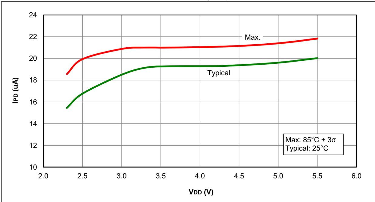
**FIGURE 27-27: I<sub>PD</sub>, BROWN-OUT RESET (BOR), BORV = 1, PIC12LF1571/2 ONLY**
