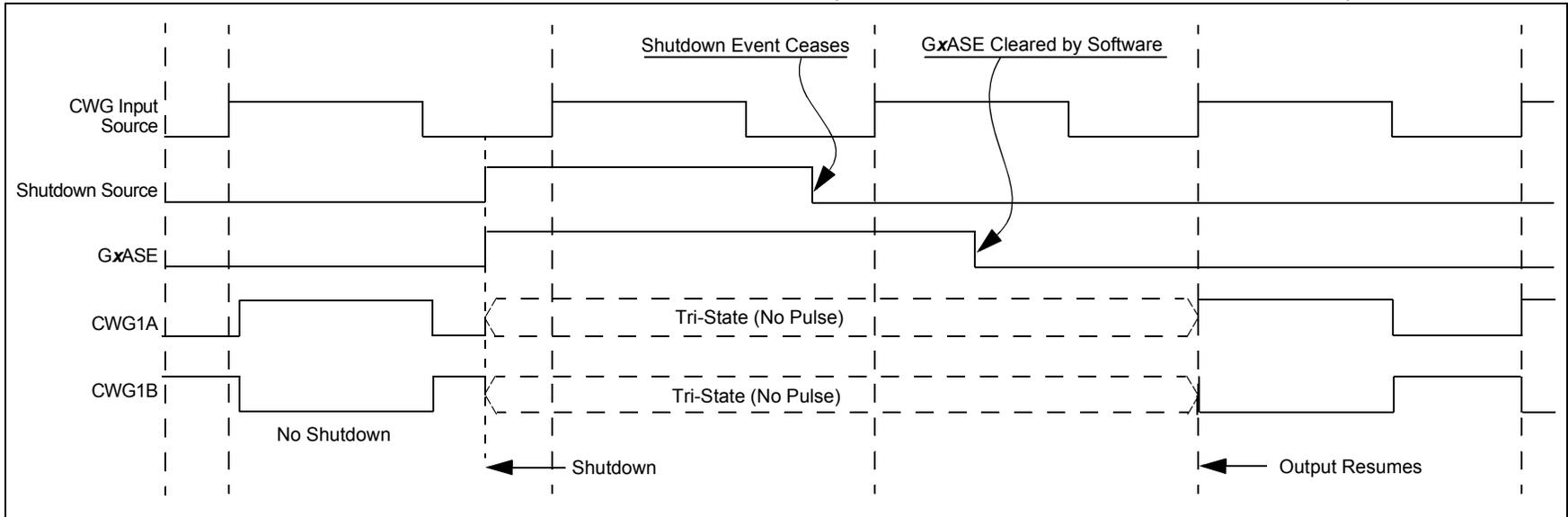
**FIGURE 23-6: SHUTDOWN FUNCTIONALITY, AUTO-RESTART ENABLED ( $GxARSEN = 1$ ,  $GxASDLA = 01$ ,  $GxASDLB = 01$ )**
