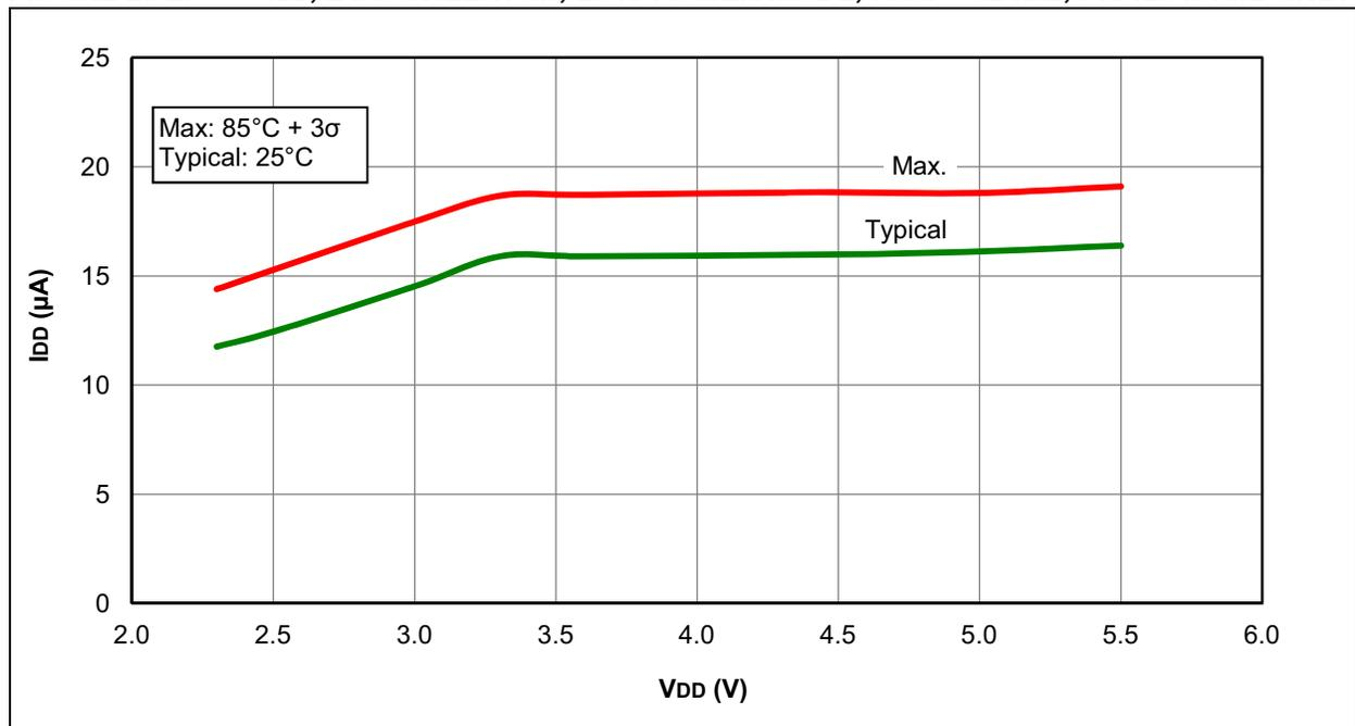
**FIGURE 27-3: I<sub>DD</sub>, EC OSCILLATOR, LOW-POWER MODE, F<sub>osc</sub> = 500 kHz, PIC12LF1571/2 ONLY**
