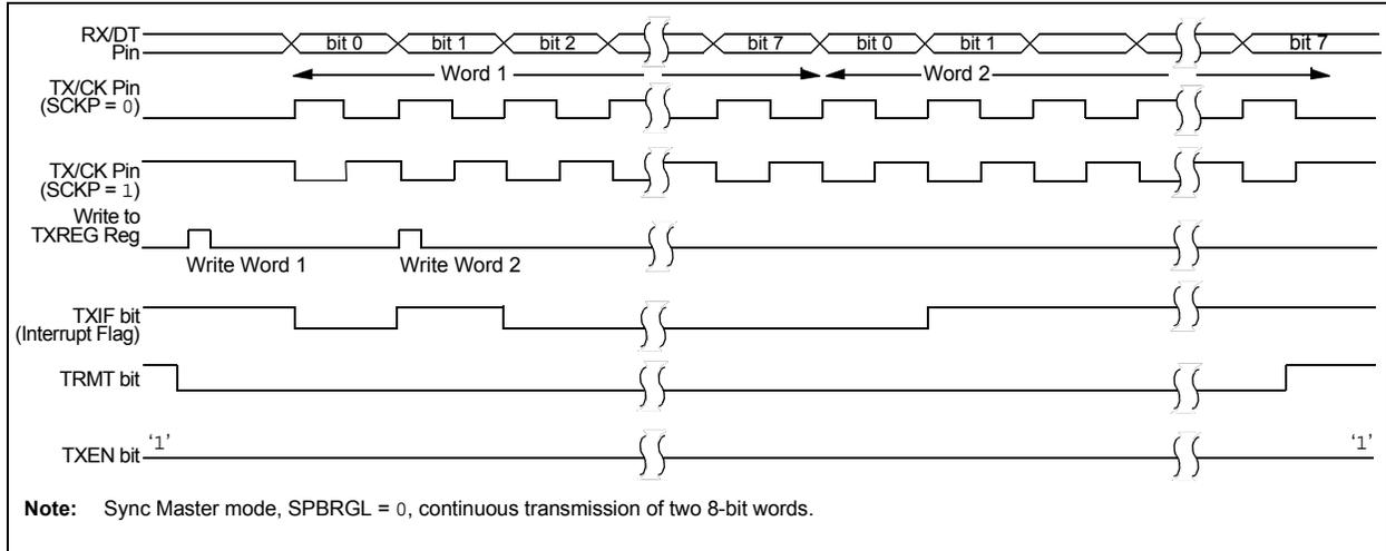
**FIGURE 21-11: SYNCHRONOUS TRANSMISSION (THROUGH TXEN)**
