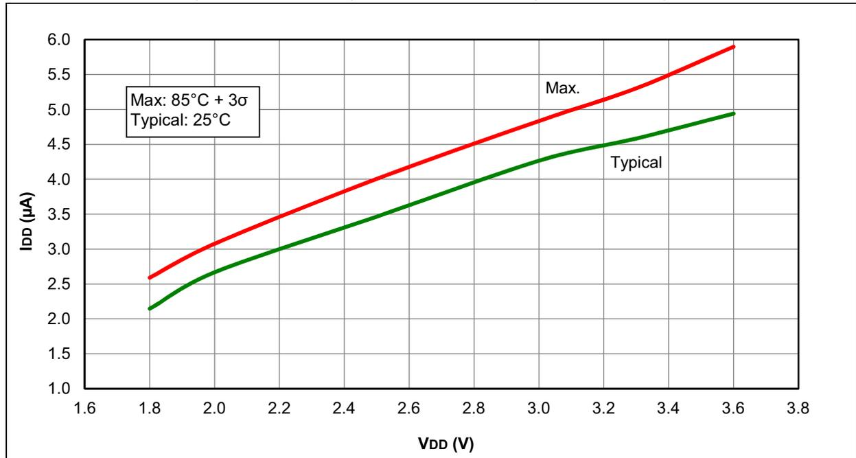
FIGURE 27-2:  $I_{DD}$ , EC OSCILLATOR, LOW-POWER MODE,  $F_{osc} = 32$  kHz, PIC12F1571/2 ONLY
