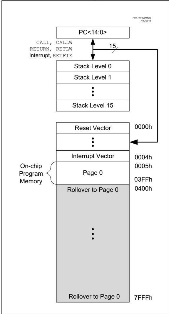
**FIGURE 3-2: PROGRAM MEMORY MAP AND STACK FOR PIC12(L)F1572**
