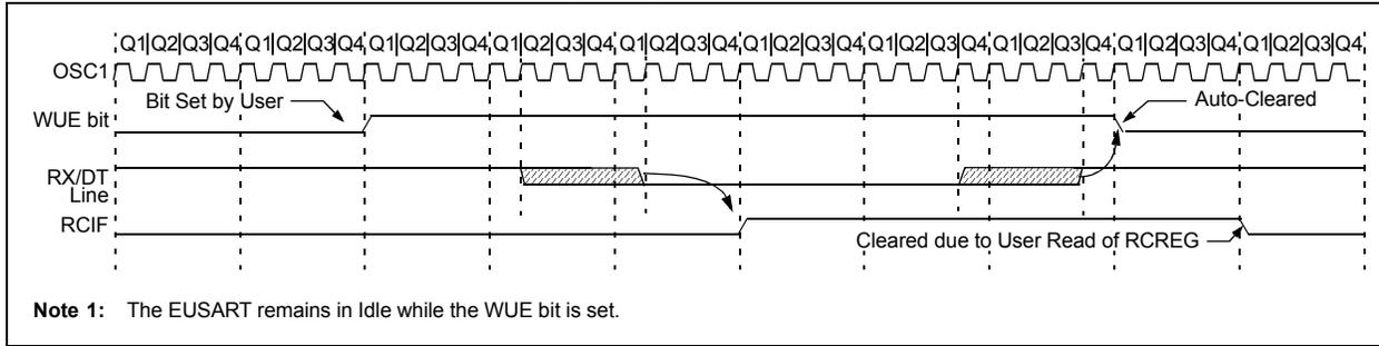
**FIGURE 21-8: AUTO-WAKE-UP BIT (WUE) TIMINGS DURING SLEEP**
