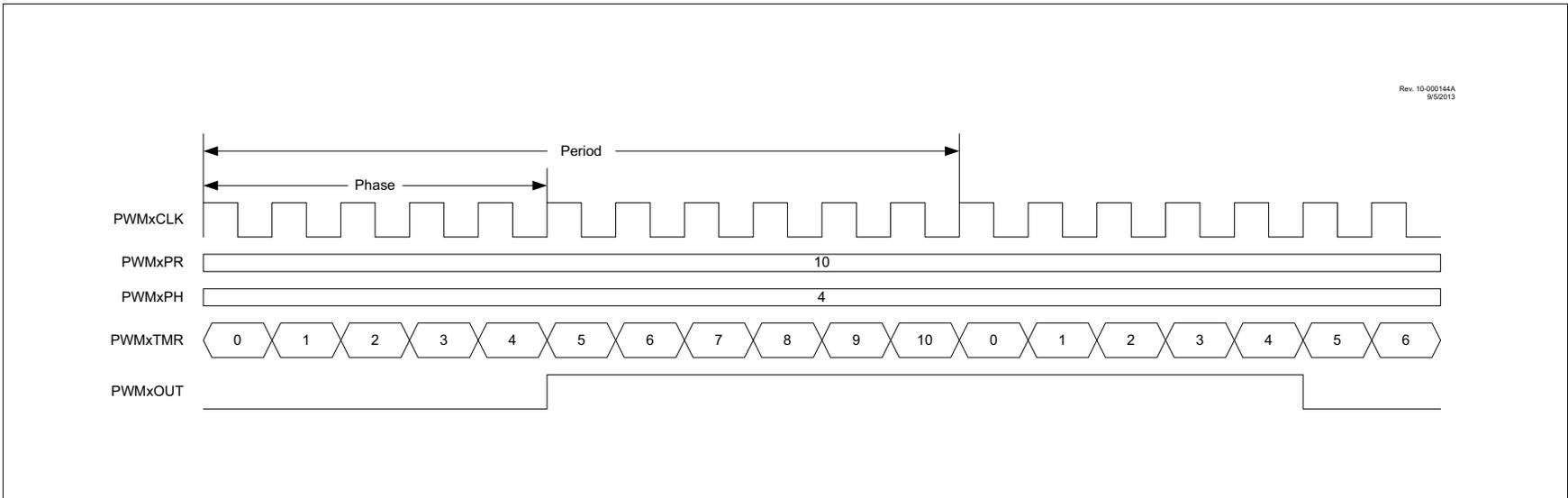
**FIGURE 22-7: CENTER-ALIGNED PWM MODE TIMING DIAGRAM**
