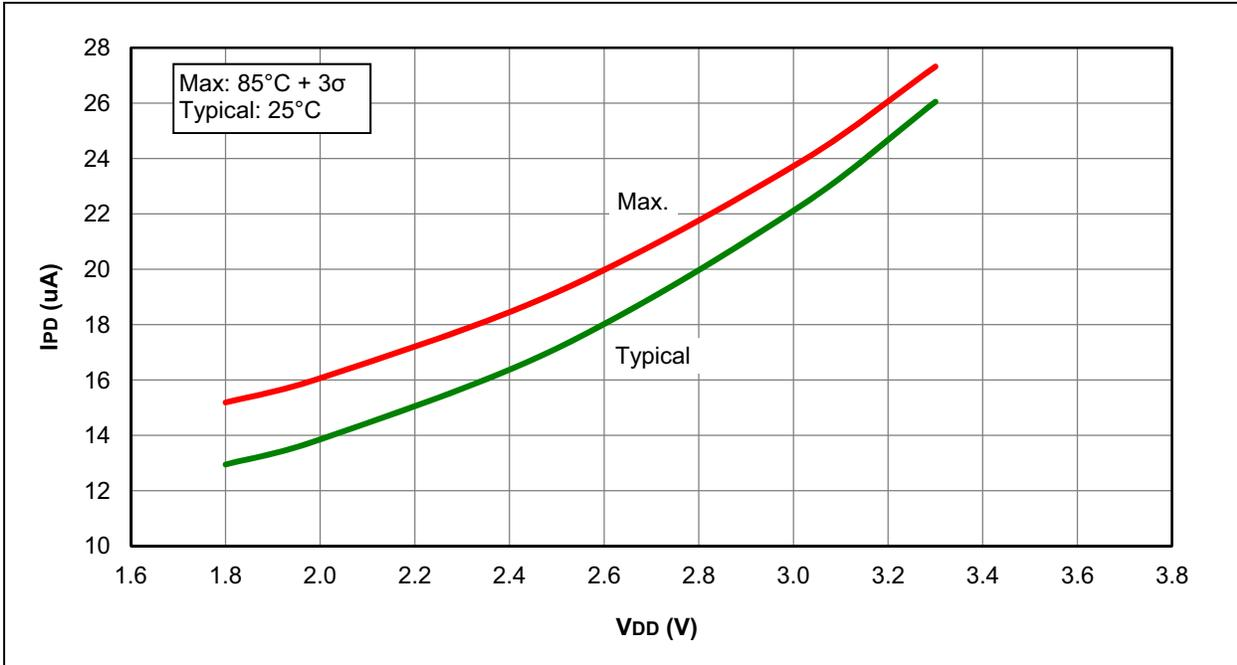
FIGURE 27-26: I<sub>PD</sub>, FIXED VOLTAGE REFERENCE (FVR), PIC12F1571/2 ONLY
