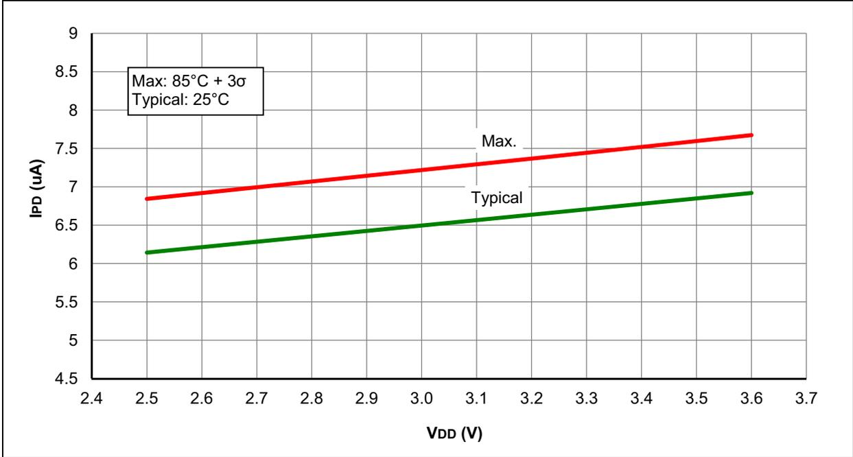
**FIGURE 27-28: I<sub>PD</sub>, BROWN-OUT RESET (BOR), BORV = 1, PIC12F1571/2 ONLY**
