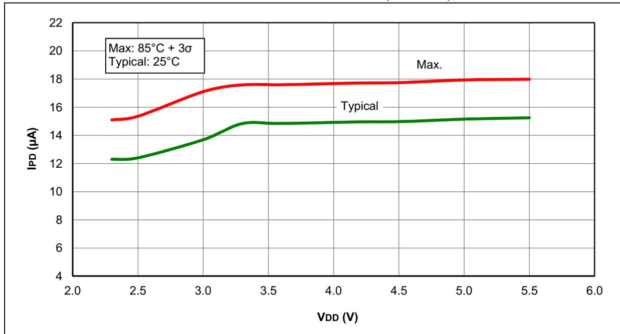
FIGURE 27-34: I<sub>PD</sub>, COMPARATOR, NORMAL POWER MODE (C<sub>x</sub>SP = 1), PIC12LF1571/2 ONLY
