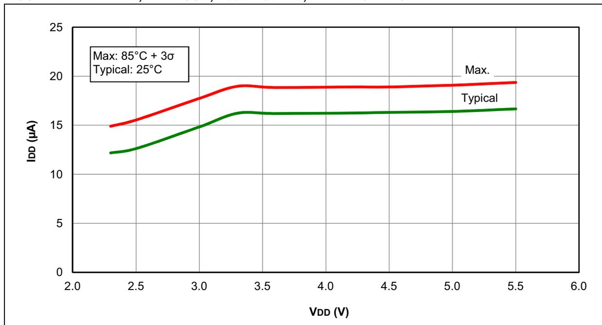
FIGURE 27-15: I<sub>DD</sub>, MFINTOSC, Fosc = 500 kHz, PIC12LF1571/2 ONLY
