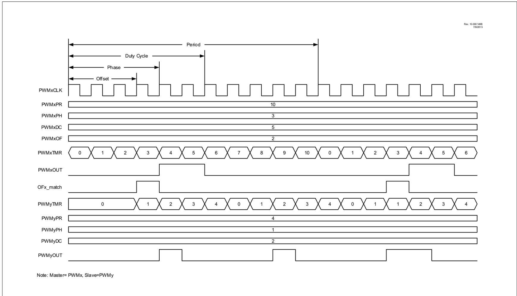
**FIGURE 22-12: OFFSET MATCH ON INCREMENTING TIMER TIMING DIAGRAM**
