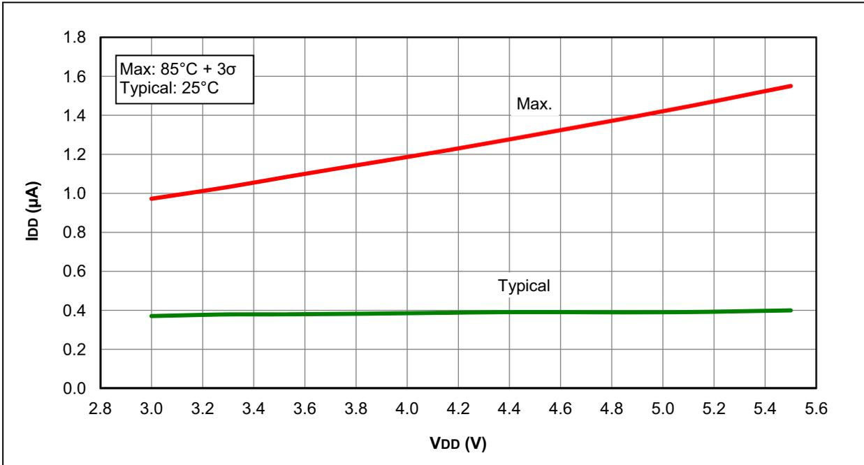
FIGURE 27-31: I<sub>PD</sub>, ADC NON-CONVERTING, PIC12LF1571/2 ONLY
