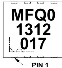
**TABLE 29-1: 8-LEAD 3x3x0.9 DFN (MF) TOP MARKING**
