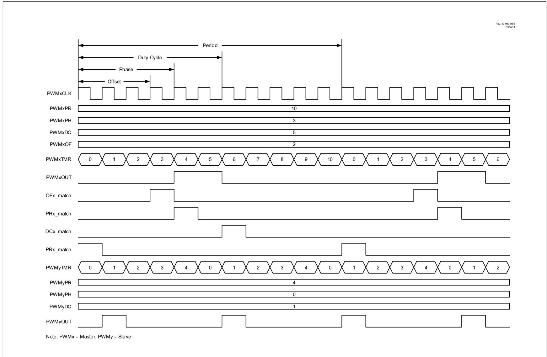
FIGURE 22-9: SLAVE RUN MODE WITH SYNC START TIMING DIAGRAM
