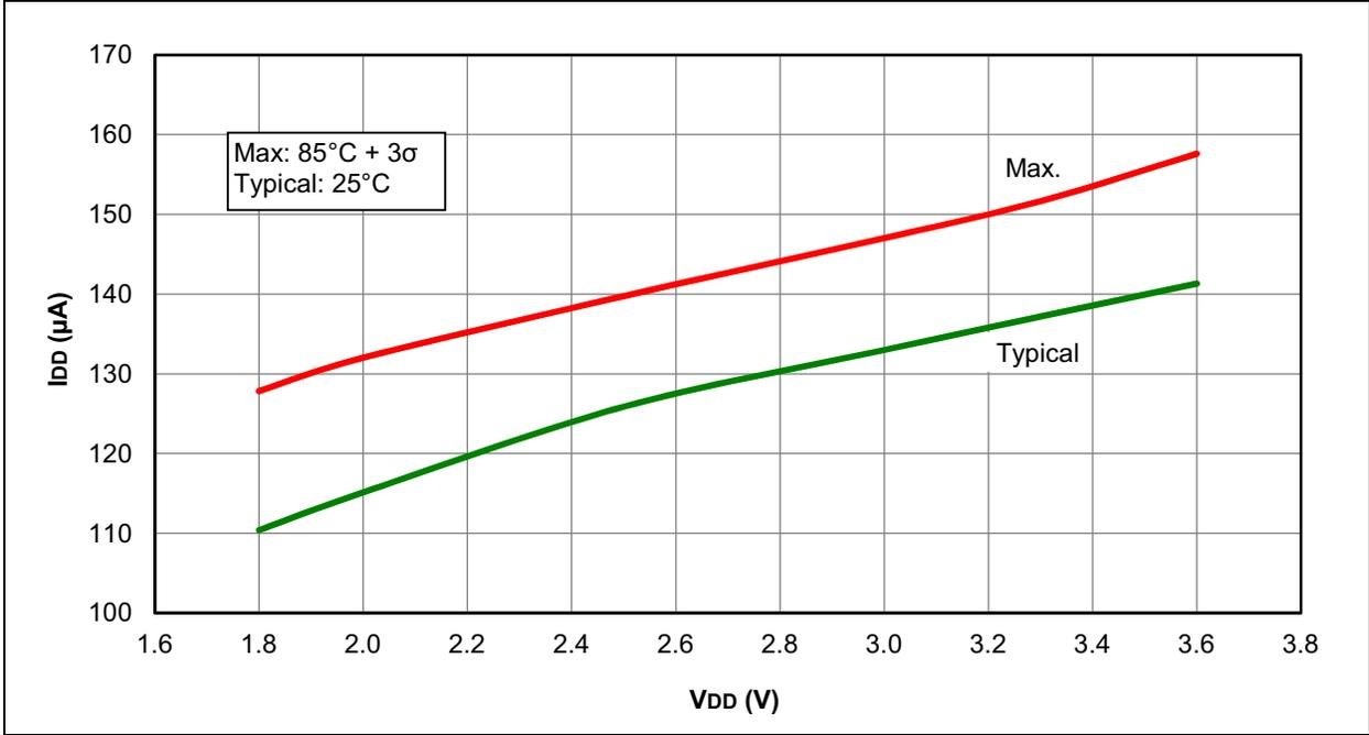
FIGURE 27-16: I<sub>DD</sub>, MFINTOSC, Fosc = 500 kHz, PIC12F1571/2 ONLY
