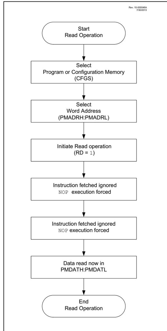
**FIGURE 10-2: FLASH PROGRAM MEMORY READ CYCLE EXECUTION**
