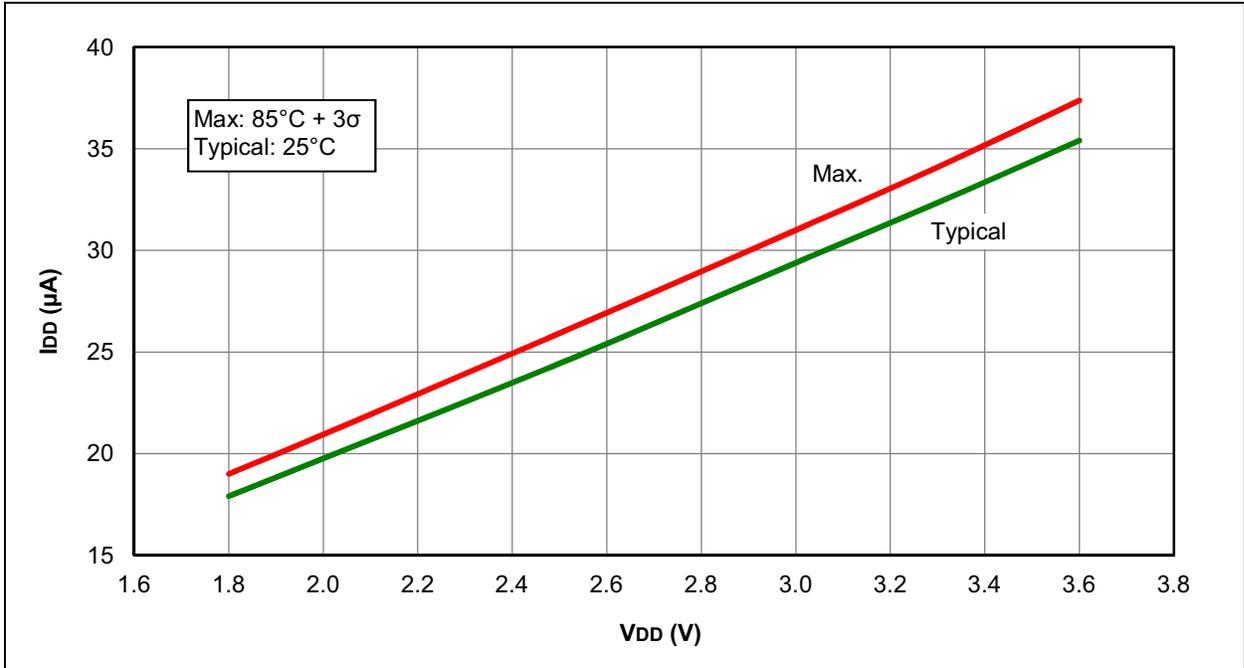
**FIGURE 27-4: I<sub>DD</sub>, EC OSCILLATOR, LOW-POWER MODE, F<sub>osc</sub> = 500 kHz, PIC12F1571/2 ONLY**
