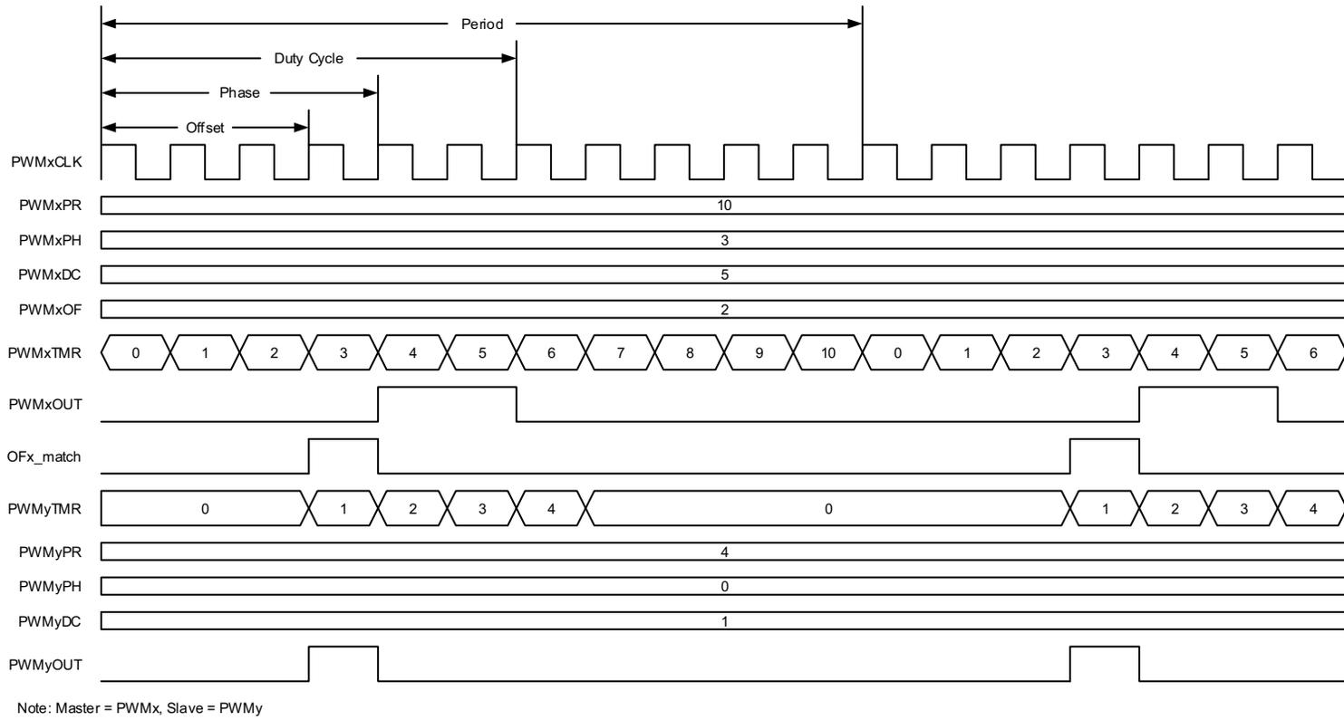
FIGURE 22-11: CONTINUOUS SLAVE RUN MODE WITH IMMEDIATE RESET AND SYNC START TIMING DIAGRAM
