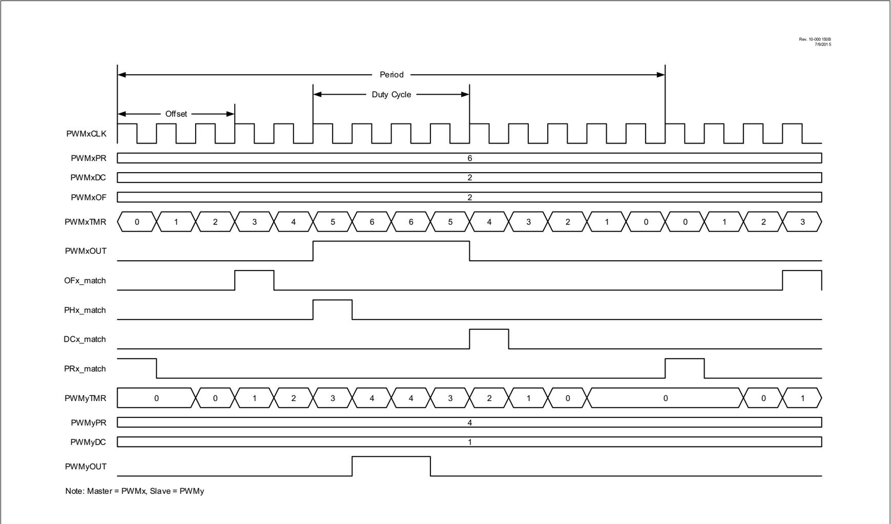
**FIGURE 22-13: OFFSET MATCH ON DECREMENTING TIMER TIMING DIAGRAM**
